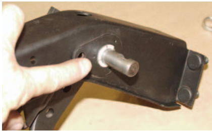
Photo #6: Before installing the new clutch arm, make sure the bushings on the clutch shaft are in good shape. If the shaft is wobbly, the bushings are bad. To replace the bushings, slide the pedal shaft out of the pivot sleeve and install two P/N 08-18 bushings. Be sure to lightly grease the bushings.
