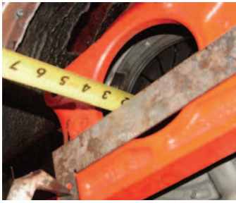
Photo #23: Next measure the distance from the face of the bellhousing to the fingers on the pressure plate. Our project car had a measurement of 2-7/8". By subtracting 2-7/8" from the 3" measurement we find that we have 1/8" (.125") clearance between the release bearing and the fingers of the pressure plate, this is within the tolerances required for the release bearing. If your measurement is not .100" to .300" turn the entire bearing assembly clockwise or counterclockwise full turns until the proper measurement is obtained.
