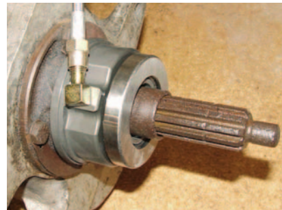
Photo #21: Next install the release bearing onto the adjusting collar by turning the bearing clockwise until the rear face of the bearing bottoms out on the front bearing retainer bolts.
