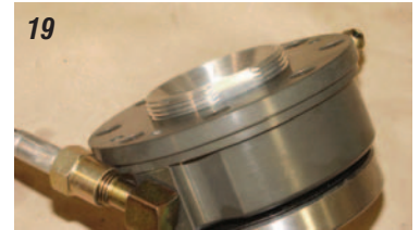
Photo #19: The release bearing is adjustable in length so that it can be used with a diaphragm or three finger type pressure plate. A set collar on the release bearing may be adjusted in or out to set the proper clearance between the release bearing and pressure plate.
