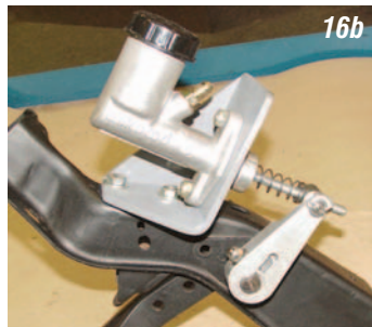
Photo #16a & 16b: Install the cotter pin and washer to hold the coupler to the clutch pedal arm. The pedal assembly is ready to be installed back under the dash.
