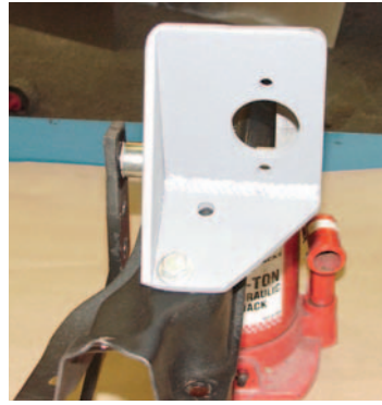
Photo #9: Bolt the bracket to the top of the pedal assembly and square up the front of the bracket to the new clutch pedal arm.
