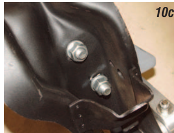
Photo #10a, 10b & 10c: Using the bracket as a guide, drill the second 3/8" hole in the pedal assembly and bolt the bracket in place.
