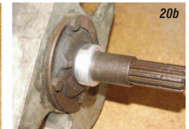
Photo #20a & 20b: The adjusting collar for the release bearing has two o-rings on the inside bore so that it will not spin. Lubricate the o-rings with a light oil and install the collar onto the front bearing retainer. The beveled side of the collar installs against the transmission face.
