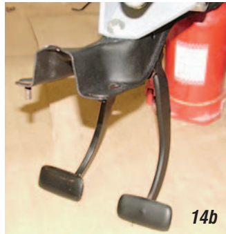
Photo #14a & 14b: The pushrod shaft for the master cylinder can be turned so that clutch pedal height can be adjusted. This can be done on the bench.
