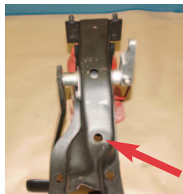
Photo #7a & 7b: Install the aluminum bushing in the kit onto the clutch arm shaft. Next install the billet aluminum clutch master cylinder arm. Make sure the offset of the arm is toward the left (driver side) of the pedal assembly. The arm is held to the shaft with an Allen head bolt and lock nut that will pass over the flat cut in the clutch pedal shaft just like the original arm.
