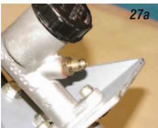
Photo #27a & 27b: The 90-degree end on the hose from the release bearing connects to the #4 fitting on the master cylinder.
