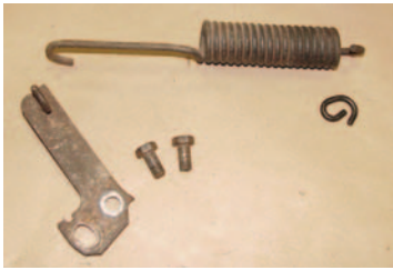
Photo #4: The stock clutch pedal swing arm has a return spring and bracket that will need to be removed. The return spring bracket is bolted to the clutch pedal arm with two 9/16" bolts.
