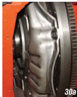
Photo #30a & 30b: Once all the air has been removed, the release bearing will move forward 1/2" to disengage the clutch. This amount of movement is enough to adequately disengage a three finger or diaphragm style pressure plate.
