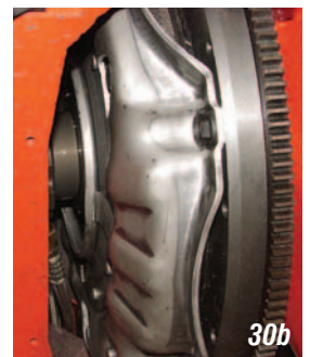
Photo #30a & 30b: Once all the air has been removed, the release bearing will move forward 1/2" to disengage the clutch. This amount of movement is enough to adequately disengage a three finger or diaphragm style pressure plate.
