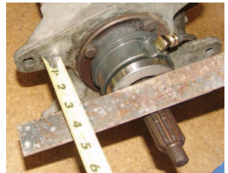
Photo #22: Measure the clearance between the release bearing and the pressure plate. To make the release bearing work properly, there must be no less than .100" and no more than .300" between the bearing and pressure plate. First measure the distance from the front of the gear box to the front of the release bearing. Our project car had a measurement of 3".
