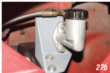
Photo #27a & 27b: The 90-degree end on the hose from the release bearing connects to the #4 fitting on the master cylinder.
