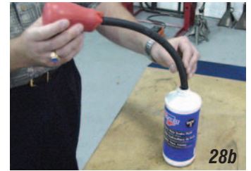
Photo #28a, 28b & 28c: With everything installed it is time to put brake fluid in the clutch master cylinder. Use ONLY DOT 3 brake fluid and not silicone brake fluid. Using silicone brake fluid will damage the release bearing and void any warranty. If the gauge cluster is removed, there is room to get a container of brake fluid up to the master cylinder top to fill the master cylinder. Fill it to within 1/2" of the top. If there is not enough room to get a container of brake up to the master cylinder use the supplied squeeze ball and hose to fill the master cylinder. Spread a garbage bag out on the floor of the car to protect the carpet.
