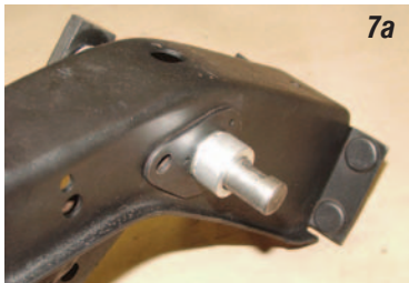
Photo #7a & 7b: Install the aluminum bushing in the kit onto the clutch arm shaft. Next install the billet aluminum clutch master cylinder arm. Make sure the offset of the arm is toward the left (driver side) of the pedal assembly. The arm is held to the shaft with an Allen head bolt and lock nut that will pass over the flat cut in the clutch pedal shaft just like the original arm.
