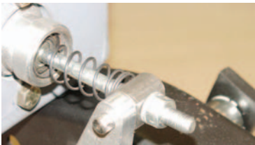
Photo #15: Once the clutch pedal height is set, lock the master cylinder pushrod to the coupler using the 5/16" fine thread nut and flat washer.
