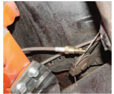
Photo #29: The clutch master cylinder will bleed just like a brake master cylinder. With the master cylinder filled, pump the pedal four or five times and hold the pedal to the floor. Now open the bleeder on the #4 hose from the release bearing allowing the air to escape. Do this several times until all the air is bled from the system.
