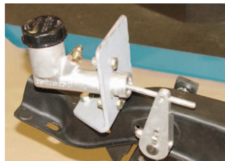
Photo #12: The clutch master cylinder bolts to the master cylinder bracket with two 5/16" X 1-1/4" bolts with lock nuts.
