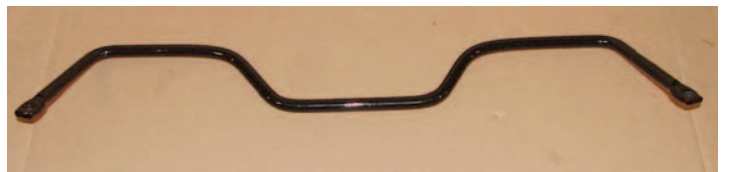
Photo 12: The rear anti-sway bar has a deep offset in the center to wrap around the center section of the rear end housing.
