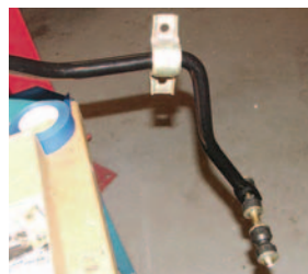
Photos 3a & 3b: The anti-sway bar is held to the bottom of the frame rails with square U-bolts and nuts, U-brackets and urethane bushings.
