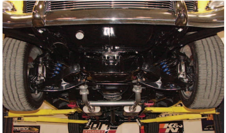
Photo 1: The front anti-sway bar mounts to the bottom of the frame rails just in front of the engine crossmember.
