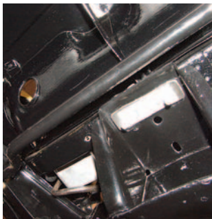
Photo 7: With the anti-sway bar in the proper location, the notched-out area in the center of the bar will clear the front mount for the radiator core support by about 3/4".
