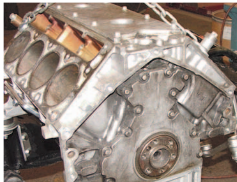
Photo #10: The back of an LS1 engine block has the same bolt pattern as an early Chevy V8 engine with one exception, there are only five bellhousing bolts instead of the normal six bolts.
