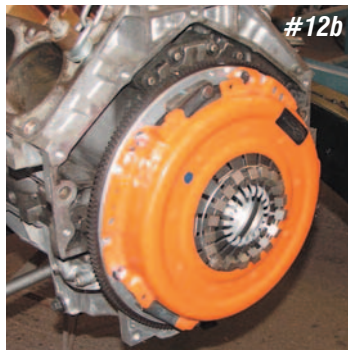
Photos #12a & #12b: We are installing the Centerforce II 11" clutch and pressure plate kit P/N 08-105. The clutch disc has 21 splines to fit the Muncie M21 or the Tremec 5-speed transmissions.
