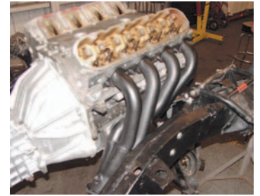
Photos #15a & #15b: Headers for the LS1 P/N 24-137 are available painted black or silver ceramic coated These headers will work with a stock steering box, 605, 670 power steering box or a CCI rack and pinion unit. The headers will not work with manual clutch linkage, so if a manual transmission is going to be used, a hydraulic clutch system must be installed. Refer to October 2006 Classic Chevy for complete instructions.
