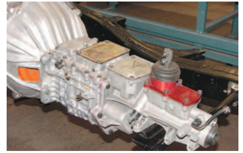
Photos #14: The Tremec 5-speed transmission P/N 08-400 is a perfect compliment for the powerful LS1 engine. The Tremec transmission bolts to the P/N 08-23
