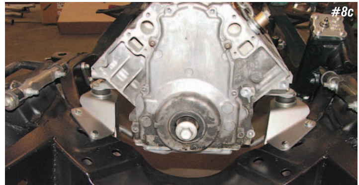
Photos #8a, #8b & #8c: With the new oil pan installed, the engine can be set down into the frame. The side engine mounts are held to the frame brackets with 7/16" x 3" bolts and lock nuts on each side. There is a large rubber grommet between the engine bracket and frame bracket and a smaller one on the bottom of the frame bracket. (See Assembly Diagram below left.)
