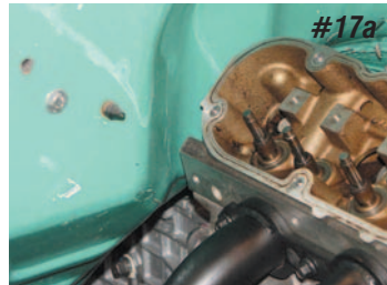
Photos #17a & #17b: Using the CCI side mount kit P/N 18-02 and adapter plates P/N18-400 to locate the LS1 engine there will be plenty of room between the back of the cylinder heads and the firewall. Installation of an automatic like a 700R4 is similar.
