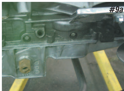
Photos #9a & #9b: You can see how much steering linkage clearance there is with the modified oil pan. The left photo shows the stock drag link and the right photo shows the rack and pinion.
