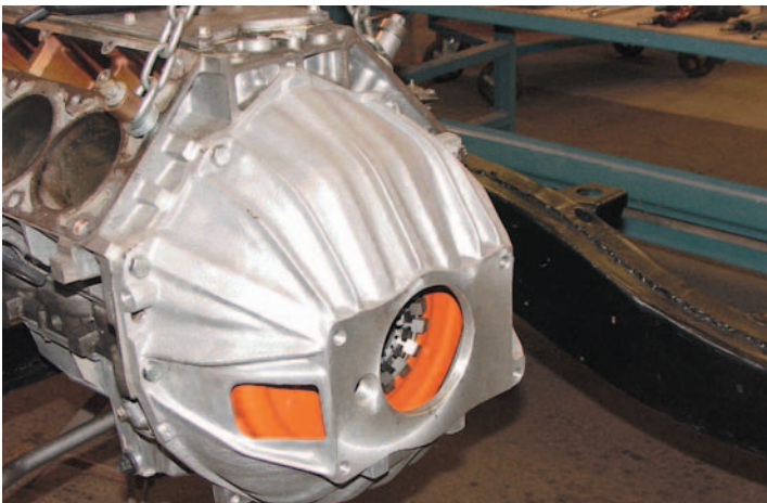
Photos #13: Along with the Centerforce II clutch kit, we are going to install an aluminum bellhousing, P/N 08-23 which is a reproduction of the late 60's early 70's big block bellhousing. The bellhousing has the standard bolt pattern that will accept a Saginaw, Muncie, Tremec or Richmond transmission and will bolt to small or big blocks and provides room for an 11" clutch.
