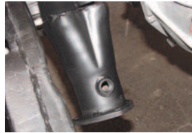
Photos #16: The driver's side header has an O2 sensor bung welded into the collector to be connected to the computer for the LS1.
