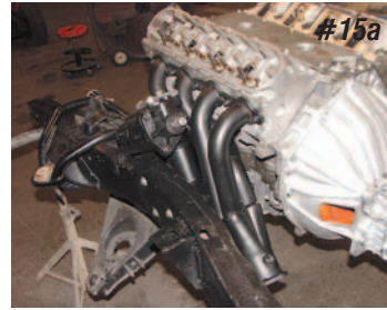
Photos #15a & #15b: Headers for the LS1 P/N 24-137 are available painted black or silver ceramic coated These headers will work with a stock steering box, 605, 670 power steering box or a CCI rack and pinion unit. The headers will not work with manual clutch linkage, so if a manual transmission is going to be used, a hydraulic clutch system must be installed. Refer to October 2006 Classic Chevy for complete instructions.
