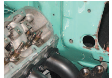
Photos #17a & #17b: Using the CCI side mount kit P/N 18-02 and adapter plates P/N18-400 to locate the LS1 engine there will be plenty of room between the back of the cylinder heads and the firewall. Installation of an automatic like a 700R4 is similar.
