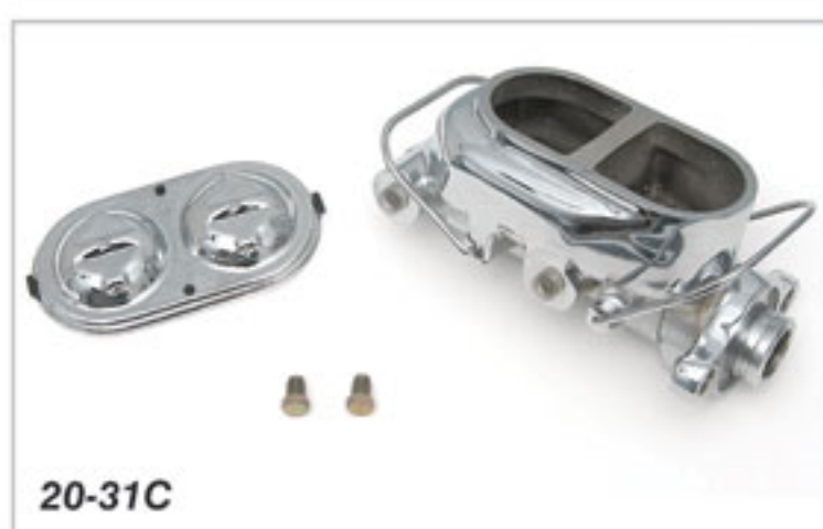
Photo #2: Not all 1968 to 72 A and F-body cars had the shallow dimple style master cylinder. Some applications used the master cylinder with the deep hole in the piston and required a booster with a long master cylinder pushrod.
