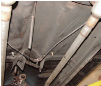
Photo #14: The cable should normally be routed under the tailpipes. Our project car has a custom exhaust system that would not allow that. With the cable connected to the linkage, adjust the linkage so that the rear emergency brakes are activated with the emergency brake handle pulled out half way.
