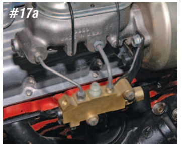
Photo #17a & 17b: The new brake like kit also includes new brake lines to be used between the brake master cylinder and the GM style proportioning valve under the hood. If your car has a dual master cylinder and the GM style proportioning valve, the front reservoir is connected to the top front port on the valve and the rear reservoir is connected to the top rear port on the proportioning valve. The new master cylinder lines are going to criss-cross the lines between the brake master cylinder and the proportioning valve. This is necessary when using the Cadillac rear calipers.
