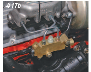
Photo #17a & 17b: The new brake like kit also includes new brake lines to be used between the brake master cylinder and the GM style proportioning valve under the hood. If your car has a dual master cylinder and the GM style proportioning valve, the front reservoir is connected to the top front port on the valve and the rear reservoir is connected to the top rear port on the proportioning valve. The new master cylinder lines are going to criss-cross the lines between the brake master cylinder and the proportioning valve. This is necessary when using the Cadillac rear calipers.
