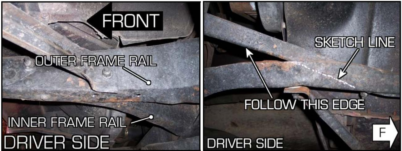
Your Hotchkis kit includes bushing bracket reinforcement plates, which will be installed on the inside of the frame rail. When measuring out where to drill the holes, your main goal is to position the holes as far forward without contacting the inner frame rails. See picture for more details. Make sure the 2 holes are parallel with the length of the car. Drill the holes using a 7/16" drill bit. Remember to always wear safety glasses when drilling.
