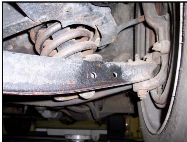
Install the end link bracket onto the lower control arm with the supplied bolts.
