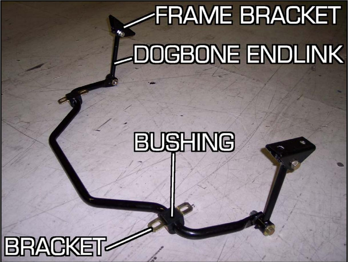
You will also need to grease the outside surface of the dogbone end link bushings. Install the end link onto the sway bar ends as shown in the picture. Use the hole closest to the end for installation purposes. Next, install the frame bracket onto the other end of the end link. The bolts do not need to be fully tight at this time, but they should be snug.
