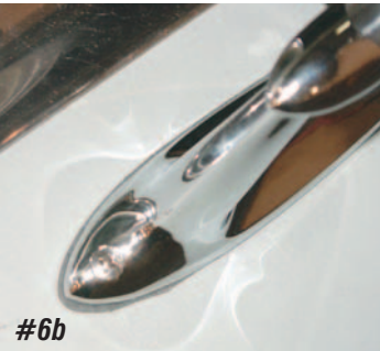
Photo #6a & 6b: Next, place the mirror on the door with the head of the #8 screw protruding into the hole in the plate on the bottom of the mirror. Slide the mirror forward, locking the mirror base to the door. Using the mirror as a guide, drill a 1/8" hole into the door for the forward mirror screw. Install the #6 countersunk screw to anchor the mirror to the door.
