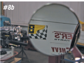
Photo #8a & 8b: Photo "A" is a shot of the shop wall about 15-feet behind our car with the stock flat glass mirror. Photo "B" is of the same wall with the new wide-angle mirror. You can see how much more area comes into your rear view with the new mirror. This will be a great safety improvement out on the road! Good luck. ✓
