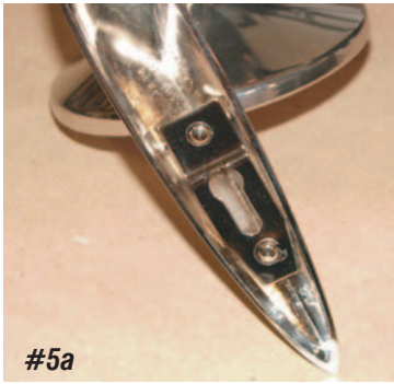
Photo #5a & 5b: On the bottom of the mirror there is a plate with a slot that will key onto the head of the #8 screw.
