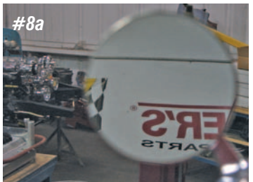
Photo #8a & 8b: Photo "A" is a shot of the shop wall about 15-feet behind our car with the stock flat glass mirror. Photo "B" is of the same wall with the new wide-angle mirror. You can see how much more area comes into your rear view with the new mirror. This will be a great safety improvement out on the road! Good luck. ✓
