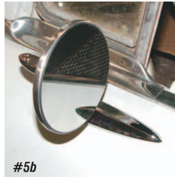
Photo #5a & 5b: On the bottom of the mirror there is a plate with a slot that will key onto the head of the #8 screw.
