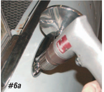
Photo #6a & 6b: Next, place the mirror on the door with the head of the #8 screw protruding into the hole in the plate on the bottom of the mirror. Slide the mirror forward, locking the mirror base to the door. Using the mirror as a guide, drill a 1/8" hole into the door for the forward mirror screw. Install the #6 countersunk screw to anchor the mirror to the door.
