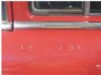
Photo #7: The locations we have given in this tech article are the exact locations that the mirror would have been installed at the dealer. We had a '57 in the shop where the customer had moved the mirror forward about 2". This made using the door mirror much easier. On a custom car, you can mount the mirrors where they work best for you.
