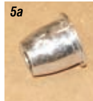
Photos 5a, 5b & 5c: Like most 1957 clusters, the chrome on the thimbles on our project car is pitted and needs to be replaced. The thimbles are included in the instrument cluster bezel kit P/N 06-69. This kit also includes the red and green lenses for the thimbles, the generator "GEN" and oil "OIL" lens and the chrome trim rings for the three gauges. Drop the new thimbles into the cluster and the green and red lenses in the appropriate thimbles.
