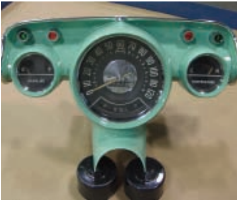
Photo 1: The 1957 instrument cluster comes out as an assembled unit. The cluster is held to the dash with four #6 sheet metal screws on the front side and two 3/8" nuts on the back side just above the steering column.
