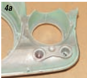
Photos 4a & 4b: At the upper left and right corners of the cluster there is a double pod socket. The outer pods have green lenses for the turn signal indicators. The inner pods have red lenses for the generator and oil warning indicators. The chrome on the thimbles that house the lenses is often pitted and the lenses may be faded and broken. The thimbles and lenses are held in with a retainers plate. The plates are held to the cluster with a single #10-32 screw on each side.
