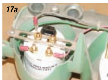
Photos 17a & 17b: Whenever possible, use the same color wires the factory used. This will make connecting to the factory dash harness much easier to do. A pink wire will need to be run from stud "I" on the two small gauges to the original pink wires that were connected to the original fuel and temperature gauges. A green wire should be connected from the "S" stud on the temperature gauge to the green wire that connected to the original temperature gauge. A tan wire will need to be connected from the "S" stud on the fuel gauge to the tan wire that connected to the original fuel gauge. Each gauge has male spade connectors for the lights. Connect a gray wire to each spade connector and connect them to the gray wires that were connected to the original gauges.
