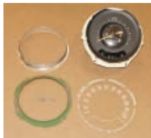
Photo 3: The speedometer is held in place with four #10-32 machine screws. Remove these four screws and the speedometer assembly can be removed from the cluster.
