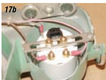
Photos 17a & 17b: Whenever possible, use the same color wires the factory used. This will make connecting to the factory dash harness much easier to do. A pink wire will need to be run from stud "I" on the two small gauges to the original pink wires that were connected to the original fuel and temperature gauges. A green wire should be connected from the "S" stud on the temperature gauge to the green wire that connected to the original temperature gauge. A tan wire will need to be connected from the "S" stud on the fuel gauge to the tan wire that connected to the original fuel gauge. Each gauge has male spade connectors for the lights. Connect a gray wire to each spade connector and connect them to the gray wires that were connected to the original gauges.
