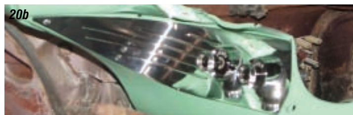
Photos 20a & 20b: The chrome dash bezels for the headlight switch, wiper switch, cigarette lighter and radio knobs are P/N 06-73. The Bel Air plastic bezel indicators P/N 06-41 fit into the chrome bezels. The headlight switch P/N 25-06 is held to the dash with the headlight switch nut P/N 06-112. We also installed the headlight switch knob and shaft P/N 06-175 and wiper switch knob P/N 06-173.
