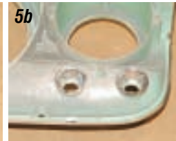
Photos 5a, 5b & 5c: Like most 1957 clusters, the chrome on the thimbles on our project car is pitted and needs to be replaced. The thimbles are included in the instrument cluster bezel kit P/N 06-69. This kit also includes the red and green lenses for the thimbles, the generator "GEN" and oil "OIL" lens and the chrome trim rings for the three gauges. Drop the new thimbles into the cluster and the green and red lenses in the appropriate thimbles.
