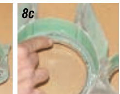
Photos 8a, 8b & 8c: The bezel kit P/N 06-69 includes two small chrome rings for the fuel gauge and temperature gauge and the large chrome ring for the speedometer. When the gauges are installed, the chrome rings are trapped between the face of the gauges and the cluster.
