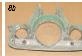
Photos 8a, 8b & 8c: The bezel kit P/N 06-69 includes two small chrome rings for the fuel gauge and temperature gauge and the large chrome ring for the speedometer. When the gauges are installed, the chrome rings are trapped between the face of the gauges and the cluster.
