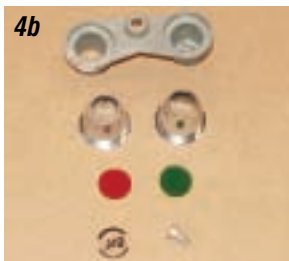
Photos 4a & 4b: At the upper left and right corners of the cluster there is a double pod socket. The outer pods have green lenses for the turn signal indicators. The inner pods have red lenses for the generator and oil warning indicators. The chrome on the thimbles that house the lenses is often pitted and the lenses may be faded and broken. The thimbles and lenses are held in with a retainers plate. The plates are held to the cluster with a single #10-32 screw on each side.
