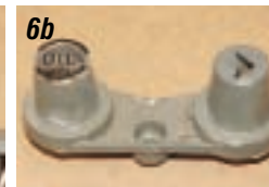
Photos 6a, 6b & 6c: The retainer plate has an arrow cut in one tower for the turn signal indicator lens while the other tower has two tabs to key the generator "GEN" or oil "OIL" indicator clear lenses.
