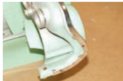
Photo 7: The cluster trim P/N 06-72 wraps around the outer perimeter of the cluster and has tabs that are bent over to hold the trim in place.
