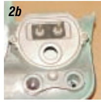
Photos 2a, 2b & 2c: The fuel and temperature gauges are held in place with two #10-32 machine screws. Remove the two screws and the gauge assembly can be removed from the cluster.
