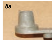
Photos 6a, 6b & 6c: The retainer plate has an arrow cut in one tower for the turn signal indicator lens while the other tower has two tabs to key the generator "GEN" or oil "OIL" indicator clear lenses.
