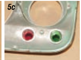
Photos 5a, 5b & 5c: Like most 1957 clusters, the chrome on the thimbles on our project car is pitted and needs to be replaced. The thimbles are included in the instrument cluster bezel kit P/N 06-69. This kit also includes the red and green lenses for the thimbles, the generator "GEN" and oil "OIL" lens and the chrome trim rings for the three gauges. Drop the new thimbles into the cluster and the green and red lenses in the appropriate thimbles.
