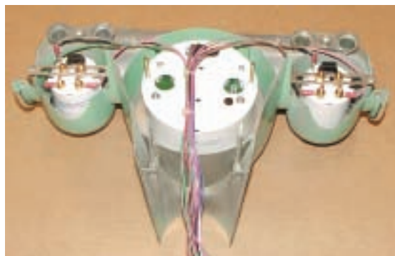
Photo 18: Using a couple of zip ties, tie all the new wires together.
