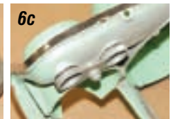
Photos 6a, 6b & 6c: The retainer plate has an arrow cut in one tower for the turn signal indicator lens while the other tower has two tabs to key the generator "GEN" or oil "OIL" indicator clear lenses.
