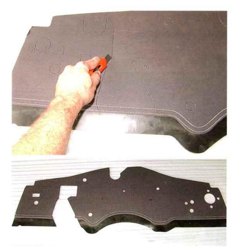
**Photo #5:** Determine which of the "punch outs" in the new insulation pad will be used in your car. If you have deleted the fresh air vents or otherwise modified the firewall, you may wish to leave some of the pre-punched areas intact. The punch-outs needed are easily trimmed out with a box knife. Also be sure to punch out all of the fastener holes.
