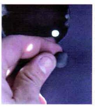
Photo #7: Using a #2 Phillips screwdriver or similar alignment tool, align each pad fastener hole with the related hole in the firewall. Holding the pad in place, insert the fasteners by hand one at a time to the first catch on the fastener. For 1955-57 cars, use tool #49-09 to push the plastic fasteners in. Do not force the fasteners all the way in just
