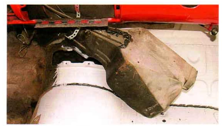
**Photo #1:** Begin by removing the front seat from the car. Also remove the glove box door, the glove box, any underdash wiring that passes through the firewall, vent and heater control cables.
