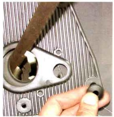
**Photo #8:** Next the appropriate rubber column seal and firewall floor seal should be slipped up over the bottom of the steering column. If the column is in the car, these two seals will need to be split with a sharp knife in order to be installed over the column. Secure theses two seals to the firewall using the five remaining fasteners.
