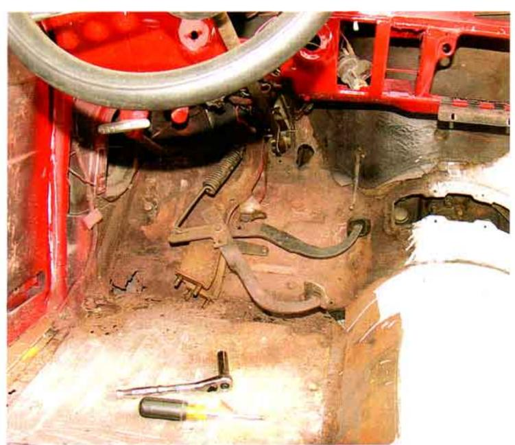
**Photo #3:** On 1955-56 cars, it will be necessary to remove the master cylinder from the firewall and the underdash swing pedal bracket as well. On 1957 cars, the insulation pad is two-pieces so these items do not need to be removed. In order to complete the job properly, the steering wheel and column should be removed from the car. You may leave these in place, but the new floor seals that will be installed will have to be cut to allow fit around the base of the column.
