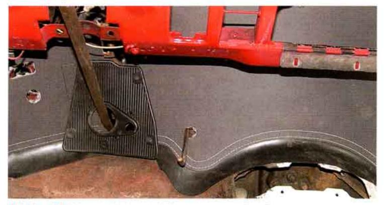
**Photo #9:** Once all the pad fasteners are in place, you may now install all of the items removed in the first few steps. The new pad will help reduce engine noise and heat inside the passenger area of your car, as well as increase the detail and value of your Classic. Good luck!
