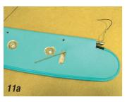
Photo #11a, 11b & 11c: The vanity lights have a two-wire harness. Using a coat hanger, pull the wires through the sunvisor material to the open corner where the sunvisor bracket mounts.
