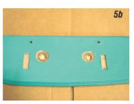
**Photo #5a & 5b:** Two 5/16" holes need to be drilled halfway through the sunvisor panel for the vanity mirror door return springs and two notches must be cut half way through the panel for the vanity mirror lights. Using the grease trick, mark the sunvisor and cut the holes and notches.
