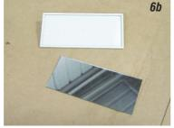
**Photo #6a & 6b:** The vanity mirror can be disassembled for painting. The mirror glass frame is flexible plastic and can be removed from the mirror assembly.
