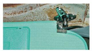
**Photo #14:** The wire for the lights may be run behind the sunvisor bracket and fed down behind the inside windshield molding. One wire needs to be connected to a good body ground and the other wire must be connected to a good constant 12-volt source. The orange wire in the dash harness that powers the dome lights works great as a 12-volt source.
