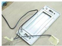
Photo #8a & 8b: The lights for the vanity mirror snap into the back side of the mirror housing. Remove the lights and cover them with masking tape so that no paint gets on the light bulbs.
