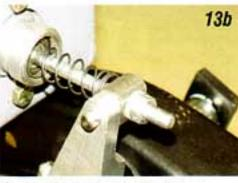
Photo #13a & 13b: The master cylinder is equipped with a threaded pushrod. The 3" long spring provided should be installed onto the pushrod shaft first. Screw the coupler onto the shaft to connect the master cylinder pushrod to the clutch pedal arm. Make sure the flat side on the coupler is facing away from the master cylinder.
