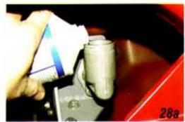
Photo #28a, 28b & 28c: With everything installed it is time to put brake fluid in the clutch master cylinder. Use ONLY DOT 3 brake fluid and not silicone brake fluid. Using silicone brake fluid will damage the release bearing and void any warranty. If the gauge cluster is removed, there is room to get a container of brake fluid up to
