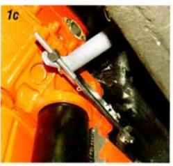
works fine when everything is in good condition, but once one part starts to wear the complete system can become sloppy. The clutch linkage also eats up a lot of engine compartment room which can limit your choice of headers.
