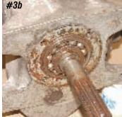
**Photo #3a & 3b:** To remove the bearing retainer, first bend the tabs back on the bolt retaining plates and remove the four bolts. Using a plastic mallet, tap on the neck of the retainer and the retainer will break free from the transmission.
