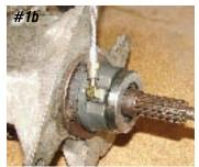
**Photo #1a & 1b:** The old universal style release bearing fit onto the stock front bearing retainer. It used an adjustable collar that screwed into the bearing. This collar was used for setting the bearing to pressure plate clearance.
