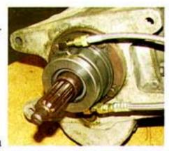
60" long #4 Teflon steel braided hose that connects the release bearing to the clutch master cylinder. Connect the straight end of the #4 hose to the lower fitting on the release bearing.
