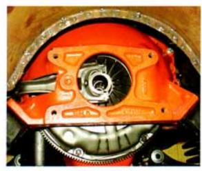
Photo #2: The clutch fork fits through a hole in the bell housing on the driver's side and connects to the mechanical release (throw out) bearing. The new hydraulic clutch system eliminates all of the clutch linkage, clutch fork and release bearing.
