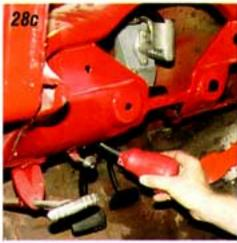
the master cylinder top to fill the master cylinder. Fill it to within 1/2" of the top. If there is not enough room to get a container of brake up to the master cylinder use the supplied squeeze ball and hose to fill the master cylinder. Spread a garbage bag out on the floor of the car to protect the carpet.
