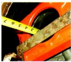
Photo #23: Next measure the distance from the face of the bellhousing to the fingers on the pressure plate. Our project car had a measurement of 2-7/8". By subtracting 2-7/8" from the 3" measurement we find that we have 1/8" (.125") clearance between the release
