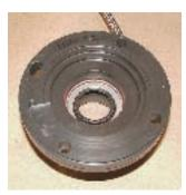
**Photo #4:** The release bearing **P/N 08-100** for a Muncie is machined to fit over the front transmission bearing and has a seal that seals to the front of the transmission. This entire assembly replaces the old bearing retainer you just removed. Each style hydraulic release bearing is custom designed to fit your
