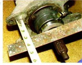
distance from the front of the gear box to the front of the release bearing. Our project car had a measurement of 3".
