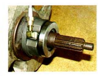
Photo #21: Next install the release bearing onto the adjusting collar by turning the bearing clockwise until the rear face of the bearing bottoms out on the front bearing retainer bolts.
