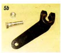
**Photo #5a & 5b:** The clutch pedal pushrod arm is splined to the clutch pedal shaft and secured with a 9/16" bolt, nut and lock washer. The stock arm will be replaced with a new billet arm for the hydraulic master cylinder.
