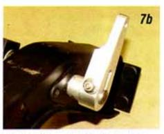
Photo #7a & 7b: Install the aluminum bushing in the kit onto the clutch arm shaft. Next install the billet aluminum clutch master cylinder arm. Make sure the offset of the arm is toward the left (driver side) of the pedal assembly. The arm is held to the shaft with an Allen head bolt and lock nut that will pass over the flat cut in the clutch pedal shaft just like the original arm.
