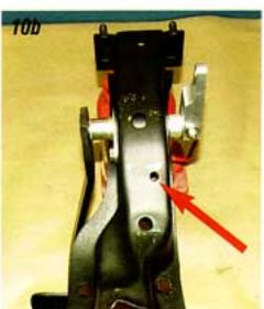
Photo #10a, 10b & 10c: Using the bracket as a guide, drill the second 3/8" hole in the pedal assembly and bolt the bracket in place.
