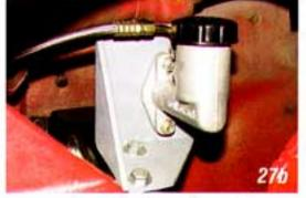
Photo #27a & 27b: The 90-degree end on the hose from the release bearing connects to the #4 fitting on the master cylinder.
