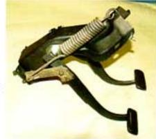
be drilled and on 1957 cars two holes must be drilled in the brake pedal swing arm assembly. To complete this, the assembly will need to be unbolted and removed from the car.
