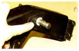
slide the pedal shaft out of the pivot sleeve and install two P/N 08-18 bushings Be sure to lightly grease the bushings.
