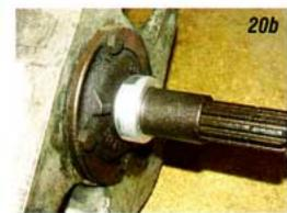
Photo #20a & 20b: The adjusting collar for the release bearing has two o-rings on the inside bore so that it will not spin. Lubricate the o-rings with a light oil and install the collar onto the front bearing retainer. The beveled side of the collar installs against the transmission face.
