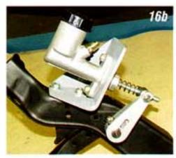
Photo #16a & 16b: Install the cotter pin and washer to hold the coupler to the clutch pedal arm. The pedal assembly is ready to be installed back under the dash.
