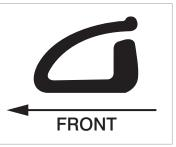
Photo #2 & Diagram: The narrow edge of the cowl weatherstripping faces to the front of the car while the open side faces to the rear.
