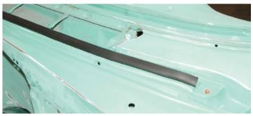
Photo #6: Snap the two fingers on the butterfly clip into the first hole in the cowl. Now do the next hole and work your way across the cowl. If the seal is too long, trim the ends with your scissors or a razor blade until even. The new weatherstripping really looks great and will keep the water and dirt away from your engine. Good Luck.
