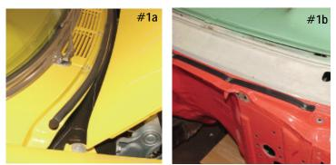
Photo #1a & 1b: The cowl weatherstripping on a 1955 and 1956 is a split rubber seal and is attached to the cowl with clips hidden underneath the flap of the seal. The cowl weatherstripping on a 1957 is a rectangular flat seal and is held to the cowl with sheet metal screws and plates.
