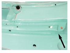
Photo #4: The cowl weatherstripping starts and ends at the end on the raised shelf on the top of the cowl.
