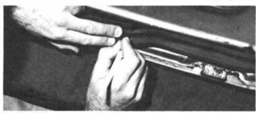
15. Carefully measure and mark the exact location for the end of the weatherstrip. Do not stretch the weatherstrip when determining where to cut because the weatherstrip will "spring" back, leaving it too short. If anything, cut the weatherstrip 1/16-inches too long. Use something very sharp, such as an X-acto knife or a razor blade to cut the weatherstrip. Make the cut so that the ends will join without leaving any gap between them.
