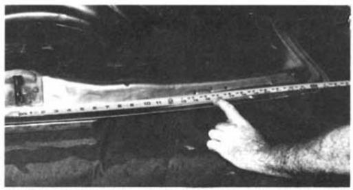
24. After consulting the diagram on page 7 for the correct orientation of the weatherstrip, start to install the weatherstrip so that the first clip to be installed is in one of the two holes with the odd spacing. The normal spacing is about 4 inches, the odd spacing was 2 ½ inches.
