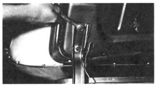
2. Scribe the location of the hinge straps on the lid inner panel. This will be a big help when it comes time to reinstall the trunk lid.
