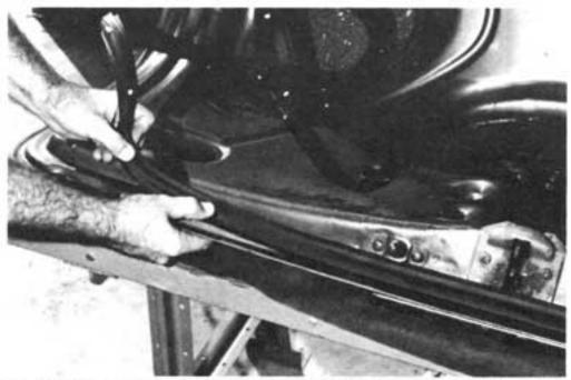
26. Continue to install the weatherstrip around the trunk lid. 27. If there is one spot where the weatherstrip puckers up due to an excessive gap between clips, a small amount of adhesive can be used to pull the weatherstrip into place.
