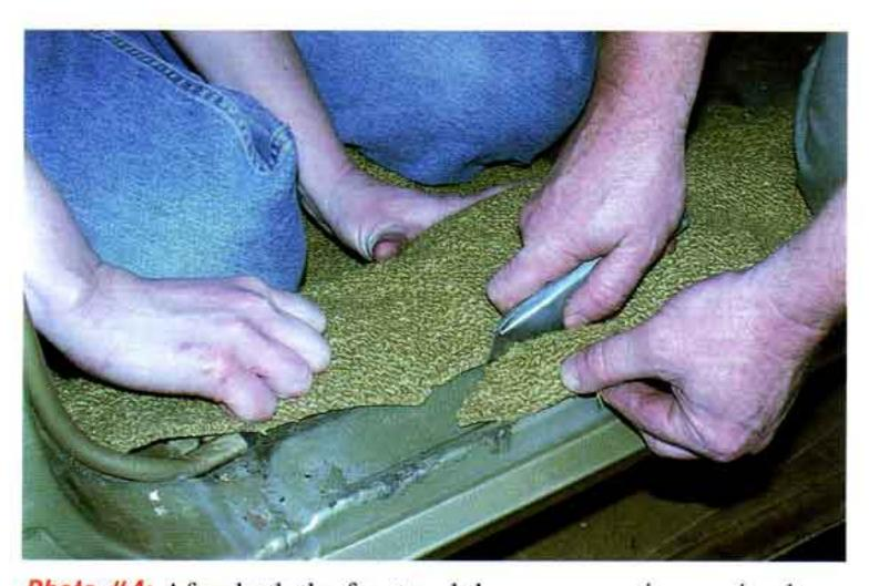
Photo #4: After both the front and the rear carpeting are in place and all holes are located, begin trimming all edges of the carpet using heavy-duty scissors or a sharp razor knife. Note: Use Super Trim Adhesive #49-22 to hold down any spots in the carpet that do not fit properly.
