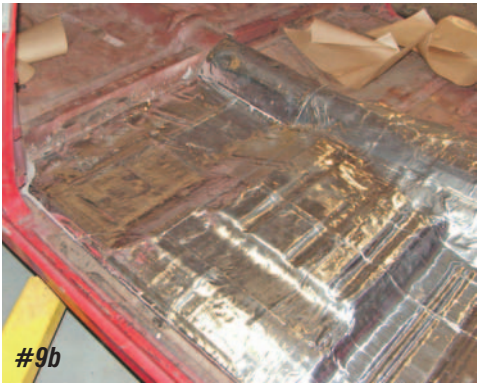
Photo #9a & 9b: Now the floor is covered completely from the firewall pad to the rear seat riser!
