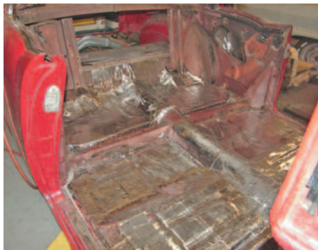
Photo #10: Using the remainder of the insulation from the floor insulation kit, cover the area under the rear seat.
