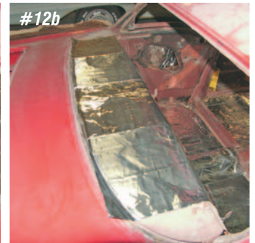
Photo #11a & 11b & 11c & 11d & Diagrams: The door and quarter insulation kit P/N 14-78 includes ten 12" X 24" tiles to cover the inner skin of the doors and quarter panel area at the quarter window. The insulation must be applied to the inside surface of the outer skin. We found it easiest to pass the tiles down through the door glass opening since there was no glass in our car. If the glass is in your car, the tiles can be folded and passed through the door access panels.
