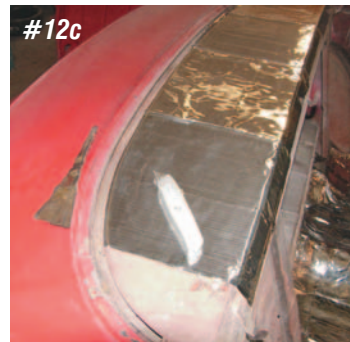
Photo #12a & 12b & 12c & 12d & 12e: The package area is another good place to install insulation. Insulating this area will keep out all of the noise and heat transferred from the trunk area. The package tray insulation kit P/N 14-80 includes four 12" X 12" tiles. This amount of material will cover about 90% of the package tray area. We had some extra material left over from the floor kit so we covered the remainder of the package tray area for 100% coverage. Using a carpet knife, we trimmed around the back glass area and around the speaker holes.
