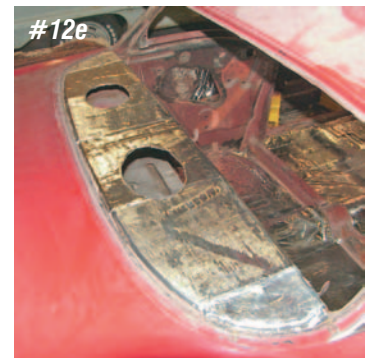
Photo #12a & 12b & 12c & 12d & 12e: The package area is another good place to install insulation. Insulating this area will keep out all of the noise and heat transferred from the trunk area. The package tray insulation kit P/N 14-80 includes four 12" X 12" tiles. This amount of material will cover about 90% of the package tray area. We had some extra material left over from the floor kit so we covered the remainder of the package tray area for 100% coverage. Using a carpet knife, we trimmed around the back glass area and around the speaker holes.
