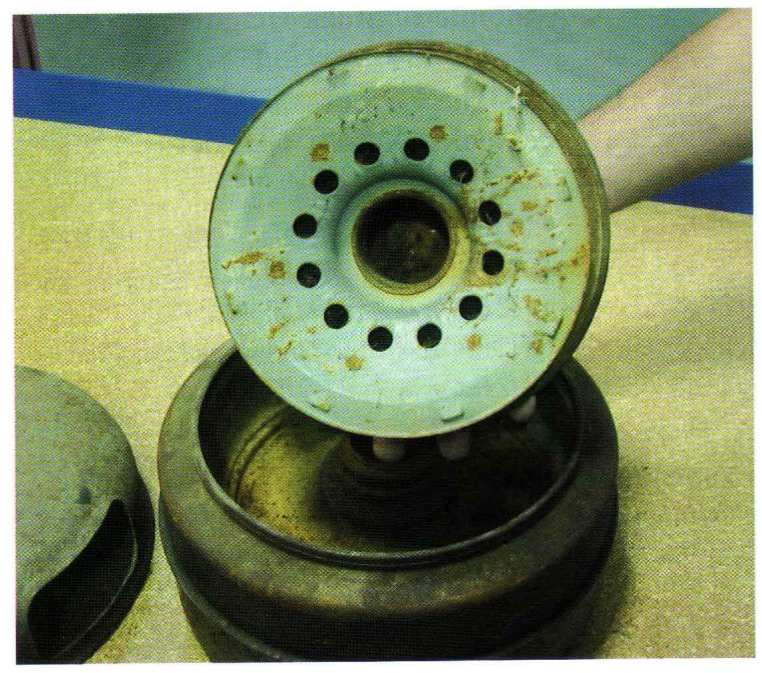
**Photo #2:** The stock filter sits down in the base of the air cleaner and has oil in the base to collect any dust/dirt that passes through filter.
