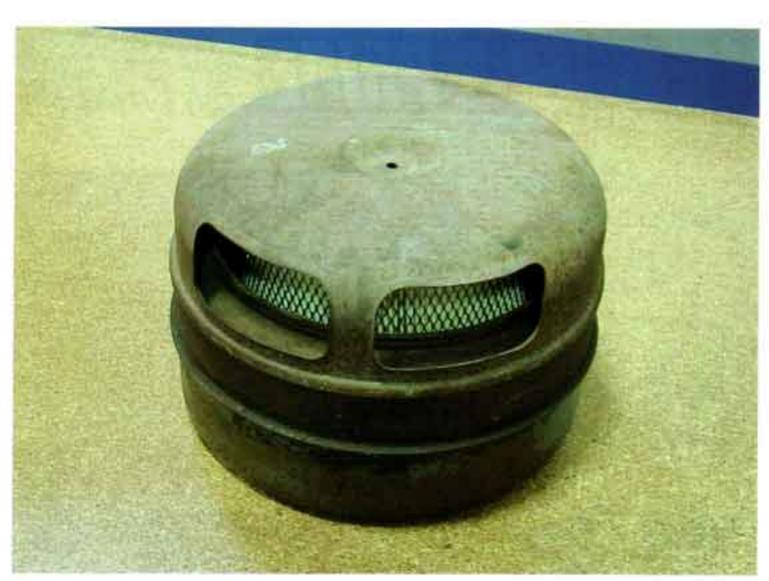
Photo #4: The stock top cover fits right over the new element. When the wing nut is tightened, the new filter will seal to the top and bottom of the air cleaner. For 1955 4-barrel air cleaners, you will need the remove the inner snorkle that protrudes into the filter cavity. Use an air cut-off wheel to remove this extra metal.
