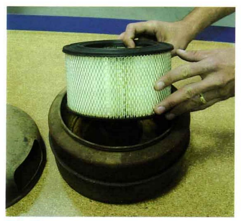
**Photo #3:** Using some rags and mineral sprits clean all the old oil out of the base of the air cleaner. The new replacement element #18-275 will sit down in the base of the stock air cleaner and center up perfectly where the stock air filter element sat.
