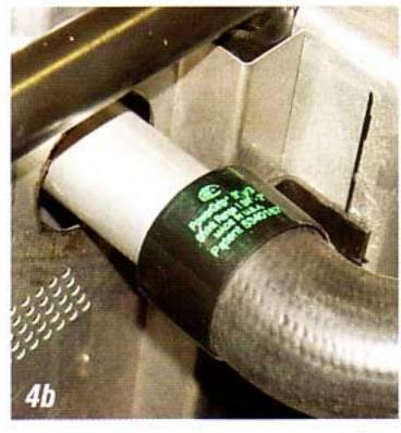
**Photo #4a & 4b:** Install the radiator hose onto the upper neck of the radiator making sure the sleeve is centered over the retaining ring flare on the radiator neck. Do not use lubricant on the hose or water neck.
