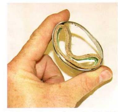
**Photo #2:** The new Powergrip sleeves come installed on a cardboard ring to keep them in shape. Remove the cardboard from the radiator hose sleeves by hand by squeezing the rings. To collapse the heater hose rings, a pair of pliers will be needed. For each end of all small or big block Chevy upper
