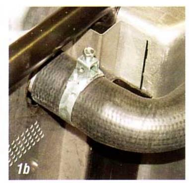
Photo #1a & 1b: A stock clamp or Gates-style hose clamp will do the job securing any hose, but when trying to clean up an engine compartment on a custom car it can take some of the smoothness away.
