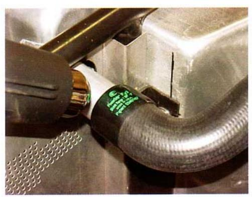
Photo #5: Using a blow dryer set on high heat or a heat gun set on medium, apply direct heat to the Powergrip sleeve. Hold the heat gun 4" to 5" from the sleeve. Do not use any kind of open flame torch to
