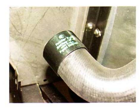
Photo #3: Once the cardboard ring has been removed, the sleeve may be installed on the end of the radiator or heater hose.
