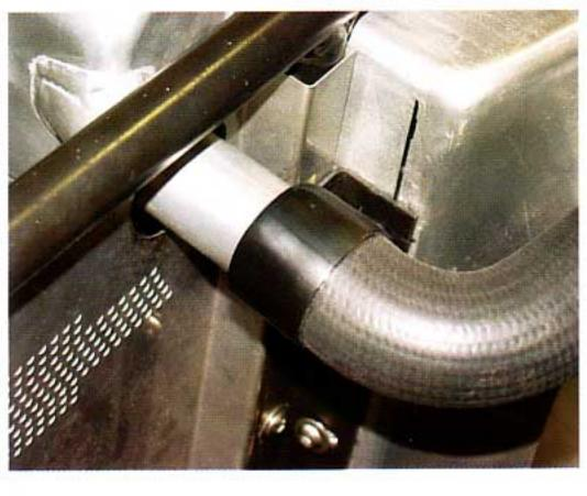
Photo #7: The green printing on the outside of the Powergrip sleeves can be removed using mineral sprits.
