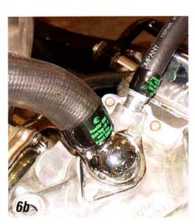
**Photo #6a & 6b:** The sleeve for the heater hoses installs the same way as the radiator hoses.
