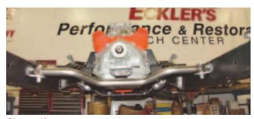
**Photo #18:** The crossmember has plenty of offset to allow any size or type of exhaust system to pass underneath.
