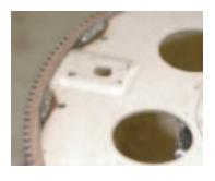
**Photo #2:** Begin by installing the TH flexplate on the engine. The automatic flexplate, **P/N 19-30**, has raised areas where the torque converter bolts on. Make sure the raised area is facing to the transmission.
