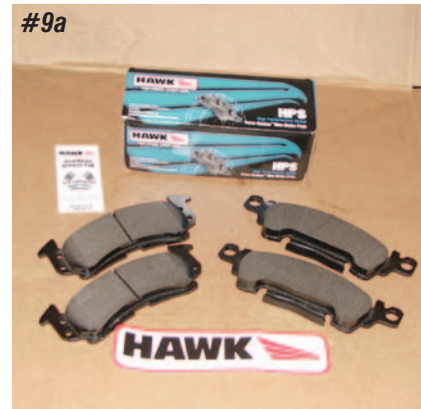
Photo #9a & 9b & 9c: The Wilwood upgrade kits P/N 20-232 and 20-233 include HAWK ceramic brake pads. These higher quality pads will give you better braking and less brake dust. There is an inner and outer pad. The pads simply drop into the jaw of the new caliper. The inner pad
