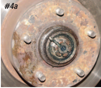
Photo #4a & 4b: Remove the dust cap, cotter pin, spindle nut and washer and the brake rotor can be removed from the spindle.
