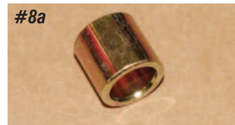
Photo #8a & 8b: The Wilwood caliper includes new anchor pins and guide sleeves. The guide sleeves install into the inner ears of the caliper housing and are held in place with O-rings. The O-rings come already installed in the caliper housing.
