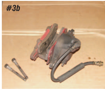
Photo #3a & 3b: Next remove the two the caliper anchor pins from the caliper and the caliper assembly and hose can be removed from the spindle.
