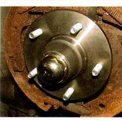
Photo #5a & 5b: Install the hub and bearing assembly onto the spindle. Pack the outer bearing with grease and install onto the spindle. Install the new spindle washer and reinstall the original spindle nut. Tighten the spindle nut to 12 ft/lbs, back it off just until it aligns with the spindle cotter pin hole. Install the cotter pins and dust covers.
