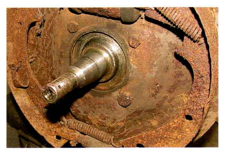
Photo #2: Clean all old grease and dirt from the spindle pin.
