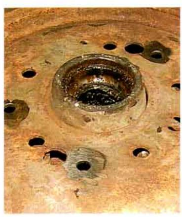
Photo #3a & 3b: If you are re-using the brake drums that were removed from the car, they will need to be separated from the original hubs. The original drum and hub assemblies were riveted together with 3 large rivets. Grind the heads off of the rivets flush with the outer surface of the brake drum. Using a large pin punch, drive the remains of the rivets out of the drum until the hub drops out.
