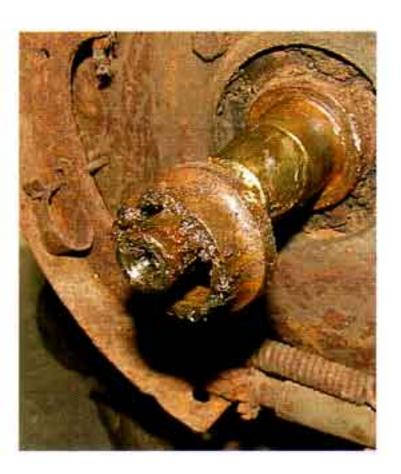
Photo #1a & 1b: Jack up the front of the car and place it on sturdy jack stands. Remove both front wheels. Remove the grease/hub dust covers, spindle cotter pin and spindle nuts. Remove both front wheel hubs and brake drums. Remove the inner bearing races from each spindle.
