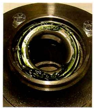
Photo #4a, 4b & 4c: Drive the new inner and outer races into the new hubs using a hammer and a flat punch. Make certain the races are driven all the way in. Grease and install the large inner roller bearing. Using a flat block of wood and a hammer, drive the inner grease seal in until flush.
