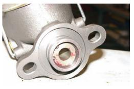
pedal push rod. A power brake master cylinder will have a shallow dimple in the piston for the brake booster push rod.
