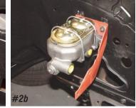
*Photo #2a & 2b:* When installing a non-power brake master cylinder, the upper two studs on the firewall are used to hold the GM style proportioning valve bracket. The lower two studs are used to hold the brake master cylinder in place.
