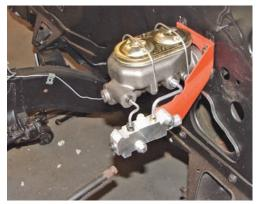
*Photo #7:* With the lines still loose, push on the proportioning valve flexing the brake lines until the holes in the valve line up with the holes in the mounting bracket and there
