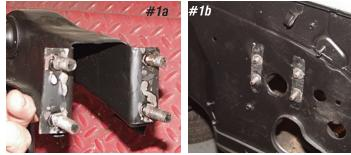
*Photo #1a & 1b:* The original master cylinder is held to the firewall with four 3/8" studs and nuts. The studs are mounted to the front of the brake pedal swing arm assembly and protrude through the four holes in the firewall.
