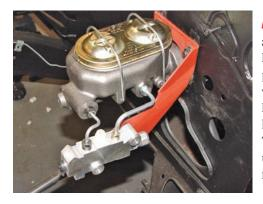
*Photo #5:* Next, attach the brake lines to the proportioning valve inlet ports leaving the nuts loose at this time. The lines will hold the valve in place for now.
