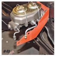
piece of cake to make them fit. When working with short, small brake lines it gets pretty tough to make them look professional if you try bending them yourself. The pre-bent lines in our kits are a nice addition. Attach the lines to the master cylinder first, leaving the nuts loose at this time.
