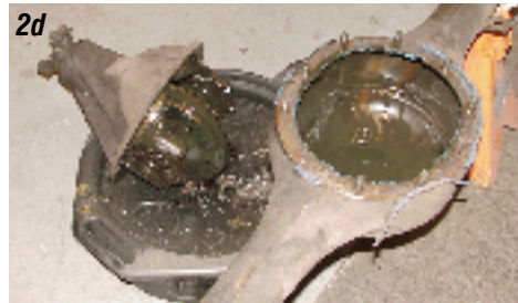
Photos 2a, 2b, 2c & 2d: To remove the center section you must first remove the axles. Remove the four backing plate bolts and the axles can be pulled out of the rear end. Next remove the ten 9/16" nuts and copper washers that hold the center section in the rear end housing. With the nuts and washers removed, a flat blade screwdriver can be used to pry the center section loose from the rear end housing.
