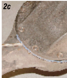
Photos 2a, 2b, 2c & 2d: To remove the center section you must first remove the axles. Remove the four backing plate bolts and the axles can be pulled out of the rear end. Next remove the ten 9/16" nuts and copper washers that hold the center section in the rear end housing. With the nuts and washers removed, a flat blade screwdriver can be used to pry the center section loose from the rear end housing.
