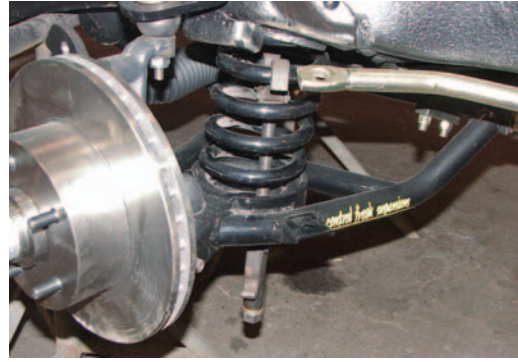
Photo #6: There is a large amount of load on the control arms when the coil spring is in place. A coil spring compressor must always be used when
