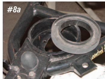
Photo #8a, 8b & 8c: If the car has tubular lower control arms, there may be a lower coil spring cushion. This cushion will need to be removed before installing the new coil-over shock conversion. On a stock lower control arm, the holes for the lower shock mount are 5/16". These holes need to be drilled out to 3/8" for the coil-over shock conversion.
