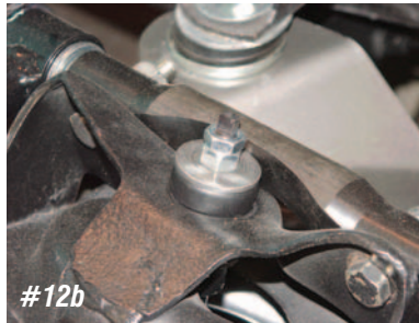
Photo #12a & 12b: The top of the QA1 shock absorber uses two washers, two rubber grommets and two nuts and attaches to the frame using the stock upper shock absorber hole.
