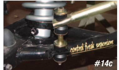
Photo #14a, 14b & 14c: With the coil-over shock installed, reconnect the outer tie rod end, the link kit for the anti-sway bar and install the brake caliper back into place.
