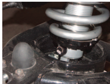
Photo #15: The dial on the QA1 coil-over shock will allow you to custom tune the dampening of the shock for your own particular taste and handling characteristics. With the dial turned all the way counter clockwise you will have a soft ride. As the dial is turned clockwise, the ride quality gets firmer and firmer all the way to "stiff."
