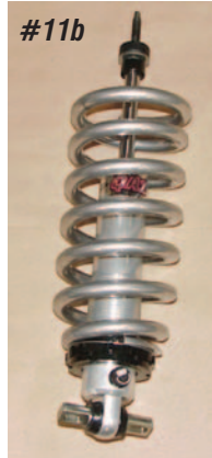
Photo #11a & 11b: The body of the shock absorber is aluminum and has threads that the spring adjusting spanner nut threads onto. By adjusting the spanner nut up or down, the ride height of the car can be set at the stock height or lowered as far as 2-7/8" from the stock height. The smaller end of the coil spring sits on top of the spanner nut.
