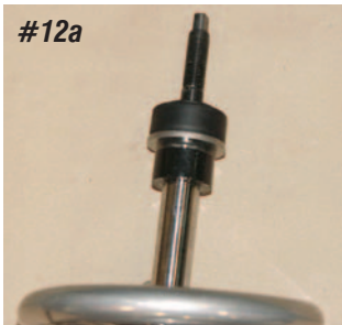
Photo #12a & 12b: The top of the QA1 shock absorber uses two washers, two rubber grommets and two nuts and attaches to the frame using the stock upper shock absorber hole.
