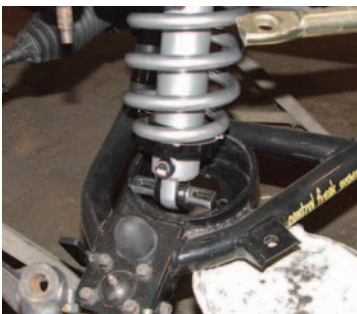
Photo #12a & 12b: The top of the QA1 shock absorber uses two washers, two rubber grommets and two nuts and attaches to the frame using the stock upper shock absorber hole.
