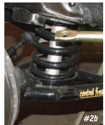
Photo #2a & 2b: To remove the coil spring, the lower control arm must be lowered out of the way. If the car has a front anti-sway bar, remove the end links that connect the sway bar to the lower control arms.
