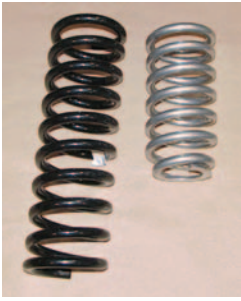
Photo #10: The top of the coil-over spring is the same diameter as a stock spring. This will allow the coil-over spring to seat in the original upper spring pocket.
