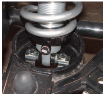
Photo #12a & 12b: The top of the QA1 shock absorber uses two washers, two rubber grommets and two nuts and attaches to the frame using the stock upper shock absorber hole.
