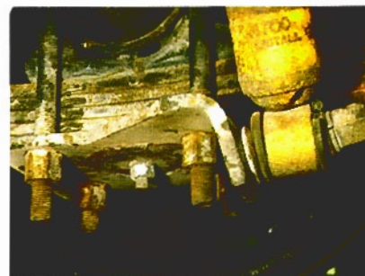
Photo #17: The rear end is held to the leaf springs with two U-bolts, nuts and a lower shock plate per side. First remove the 3/4" nut that holds the shock to the lower shock plate.
