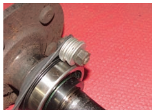
Photo 8: To install the axle retaining plate studs, simply stack up about seven or eight washers on the stud and using the backing plate nuts pull the studs into place.
