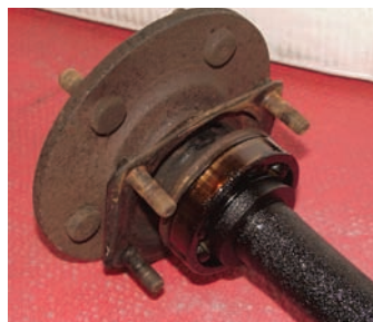
Photo 1: Remove the rear wheels, brake drums and loosen the four nuts that secure the axle retaining plate to the rear end. Using an axle puller, remove the axles from the rear end housing. The axle bearing is pressed onto the axle and is held in place with a pressed-on retaining ring.
