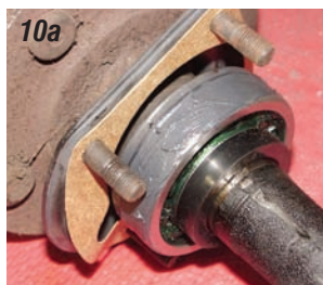
Photos 10a & 10b: Before installing the axle into the rear end, lubricate the O-ring on the outside of the bearing with a light grease to help keep the O-ring from being damaged.
