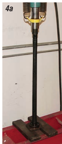
Photos 4a, 4b & 4c: A hydraulic press must be used to remove the axle bearing. Before applying any pressure to the bearing, wrap a heavy towel or rag over the bearing. If the bearing breaks while being pressed off, the towel will retain any broken pieces and help prevent any injury to you.
