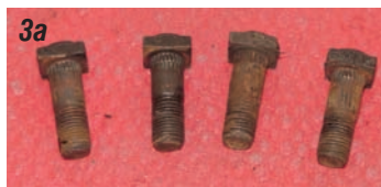
Photos 3a & 3b: The axle bearing cover has four studs that hold the axle to the rear end housing. These must be removed to allow the bearing to be pressed off. Using a hammer, tap the studs out of the bearing cover.
