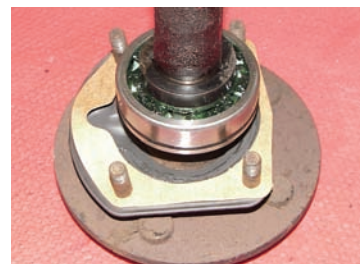
Photo 9: The gaskets used on the axle bearing cover keep any brake dust from getting to the axle bearing and damaging the bearing or seal. This seal does not retain rear end lube.
