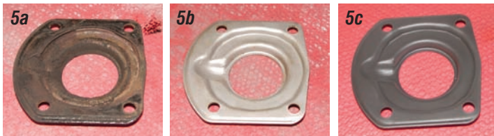
Photos 5a, 5b & 5c: The axle bearing cover has a gasket P/N 03-32 or 563206 that keeps the brake dust away from the axle bearing. These gaskets should always be replaced. We cleaned our bearing cover and painted it chassis black.
