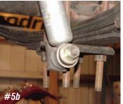
*Photo #5a & 5b:* The rear end housing is held to the leaf springs with two U-bolts on each side. The U-bolts wrap around the rear end and hold the lower shock plate in place.
