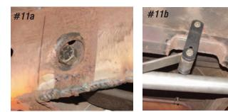
*Photo #11a & 11b:* Install the new leaf springs, leaving the front nut and bolt and shackle nuts loose at this time.
