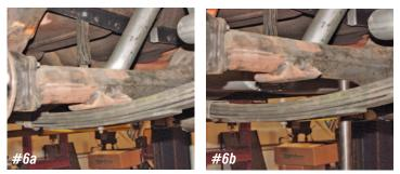
*Photo #6a & 6b:* With the frame on jack stands or the car raised on a lift, remove the shock absorber. Next remove the four nuts from the U-bolts and raise the rear end off the leaf spring one side of the car at a time.
