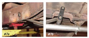
**Photo #7a & 7b:** The leaf spring is anchored to a bracket on the frame in the front with a single 1/2" bolt and to the rear of the frame with a shackle. Our project car has the CCI Spring Pocket Kit **P/N 21-131** that mounts the leaf spring parallel with the frame rails allowing for a larger tire. The removable of the leaf springs will be the same procedure as stock.
