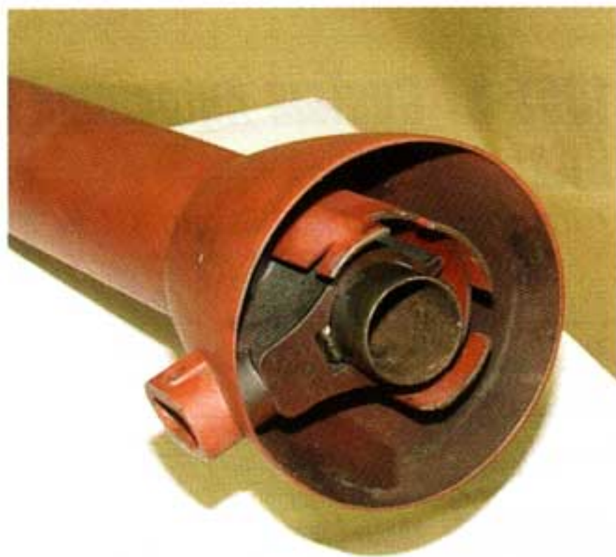
Photo #3: The shift collar will slide onto the shift tube and key into place. Use a small amount of grease on the shift tube to allow the shift collar to slide freely. Make sure the shift collar is slid down all the way.
