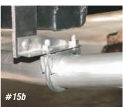
**Photo #15a & 15b:** The tailpipe hanger has a rubber strap with a steel tab to fit under the muffler clamp. Mount the hanger to the rear of the bracket and using the supplied muffler clamp, bolt the tailpipe in place. The tailpipes on the performance systems run between the rear end and the shocks while stock systems run between the shocks and the frame.
