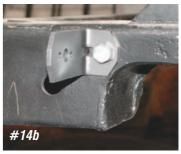
**Photo #14a & 14b:** The tailpipe hangers are held to the frame using stock dual exhaust tailpipe hanger brackets, also included in the new exhaust system. The brackets are bolted to the frame just behind the rear shackle mounts using one bolt into the frame. There are two holes in the frame; one for the mounting bolt and one for the locating tab on the bracket.
