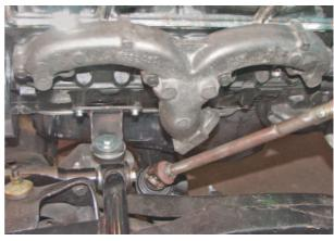
**Photo #2:** Using the 1969-72 Chevy truck rear dump rams horn manifold P/N 18-414, it will be a breeze to connect an exhaust pipe to the manifold. It looks like GM made this manifold just for our application.
