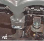
**Photo #8a & 8b:** The flat gasket included with the exhaust system seals the heat riser or heat riser delete to the exhaust manifold. With the heat riser or heat riser delete in place, install the passenger side exhaust pipe leaving the three nuts loose at this time.
