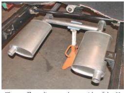
rear outlet is offset. The mufflers slip over the outside of the H-pipe with the outlets oriented toward the frame.
