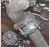
exhaust pipe and seats on the ring of the pipe for a leak-proof seal. The exhaust pipe flange includes a collar. When properly installed, the collar fits the ring on the exhaust pipe. Install the driver's side exhaust pipe to the manifold leaving the three nuts loose at this time.
