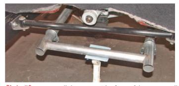
**Photo #9:** Next, install the H-pipe. The front of the H-pipe will slip up over the exhaust pipes and is held to the exhaust pipes with a muffler clamps. This fully functional H-pipe improves horsepower by equalizing the exhaust pulses as close to the engine as possible.
