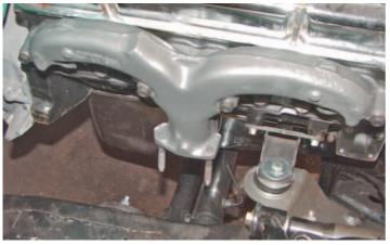
**Photo #3:** On the passenger side, there is plenty of clearance between the rack and pinion and a standard 2" center dump rams horn manifold. This manifold is readily available, used, from any early 283 or 327 or **P/N 24-297.**
