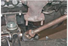
Photo #1: The coupler shaft for the rack and pinion will not allow the use of a center dump rams horn exhaust manifold on the driver's side.
