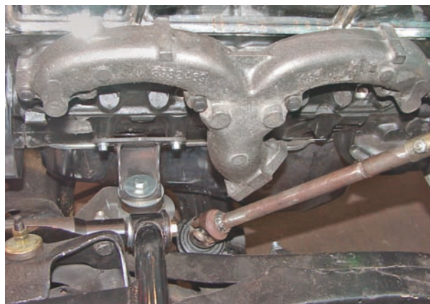
Photo #2: Using the 1969-72 Chevy truck rear dump rams horn manifold P/N 18-414 , it will be a breeze to connect an exhaust pipe to the manifold. It looks like GM made this manifold just for our application.
