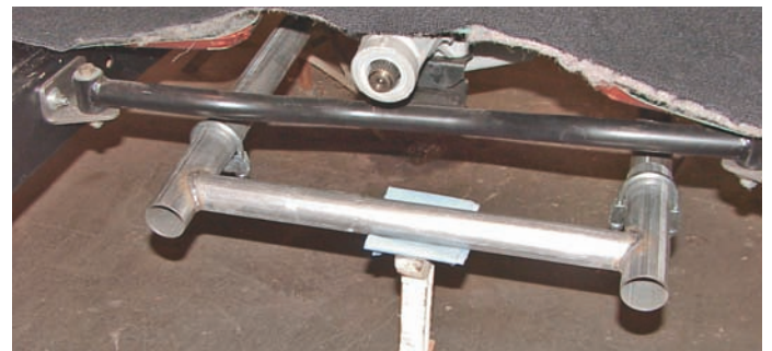
Photo #9: Next, install the H-pipe. The front of the H-pipe will slip up over the exhaust pipes and is held to the exhaust pipes with a muffler clamps. This fully functional H-pipe improves horsepower by equalizing the exhaust pulses as close to the engine as possible.
