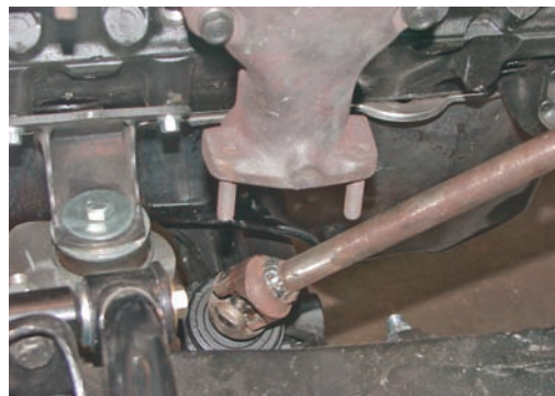
Photo #1: The coupler shaft for the rack and pinion will not allow the use of a center dump rams horn exhaust manifold on the driver's side.
