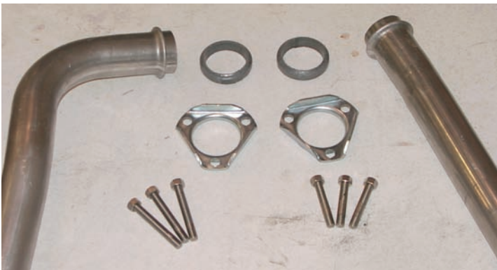
Photo #4: The exhaust system includes two donuts, one gasket for the heat riser and two flanges for the exhaust pipes. We are installing new stainless steel studs and nuts P/N 18-178 in our manifolds.
