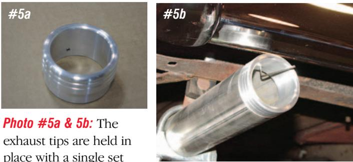
**Photo #5a & 5b:** The exhaust tips are held in place with a single set screw. Slide the tip up inside the tailpipe and orient the set screw at the top or 12:00 o'clock position. With the set screw at the top, it will be out of sight when standing behind the car. Using the supplied 5/64" Allen wrench tighten the set screw.
