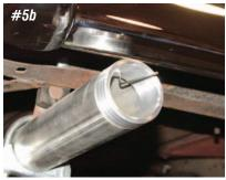
screw. Slide the tip up inside the tailpipe and orient the set screw at the top or 12:00 o'clock position. With the set screw at the top, it will be out of sight when standing behind the car. Using the supplied 5/64" Allen wrench tighten the set screw.
