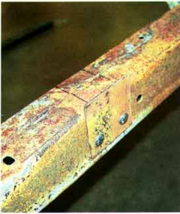
Photo #11a & 11b: Install the crossmember brackets and outer frame reinforcement plates on the frame using the 5" x 3/8" carriage bolts, washers, lockwashers and nuts included. Complete the installation by attaching the column shift linkage, TVI cable and brackets, dipstick and tube. You may now tighten all the installation hardware.
