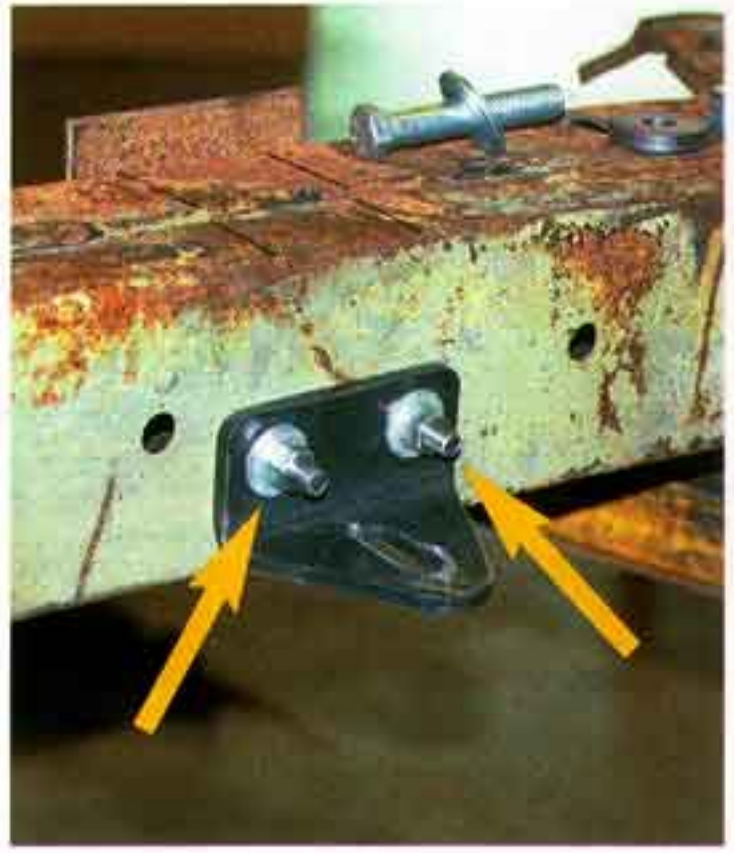
Photo #11a & 11b: Install the crossmember brackets and outer frame reinforcement plates on the frame using the 5" x 3/8" carriage bolts, washers, lockwashers and nuts included. Complete the installation by attaching the column shift linkage, TVI cable and brackets, dipstick and tube. You may now tighten all the installation hardware.
