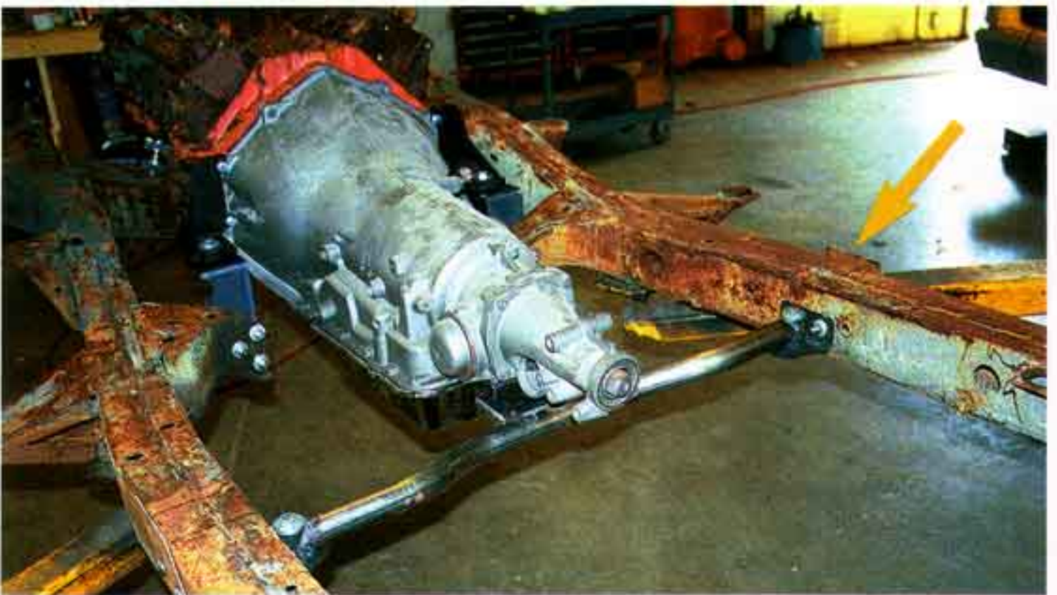
Photo #12: With the installation now complete, you will need to shorten the driveshaft to the correct length. Install the 700R4 yoke into the rear of the transmission until it hits bottom. Pull it out about 1" to 1-1/2" and measure for driveshaft length. Take the driveshaft to a local driveline shop to be shortened to the proper length.
