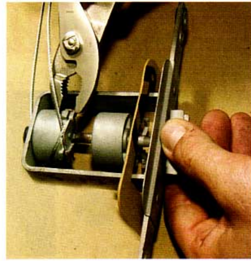
Photo #7: Once the cable is connected to the hub, squeeze the hook on the center drum slightly so that the cable cannot come loose. Don't squeeze too much or the hooks will break off.
