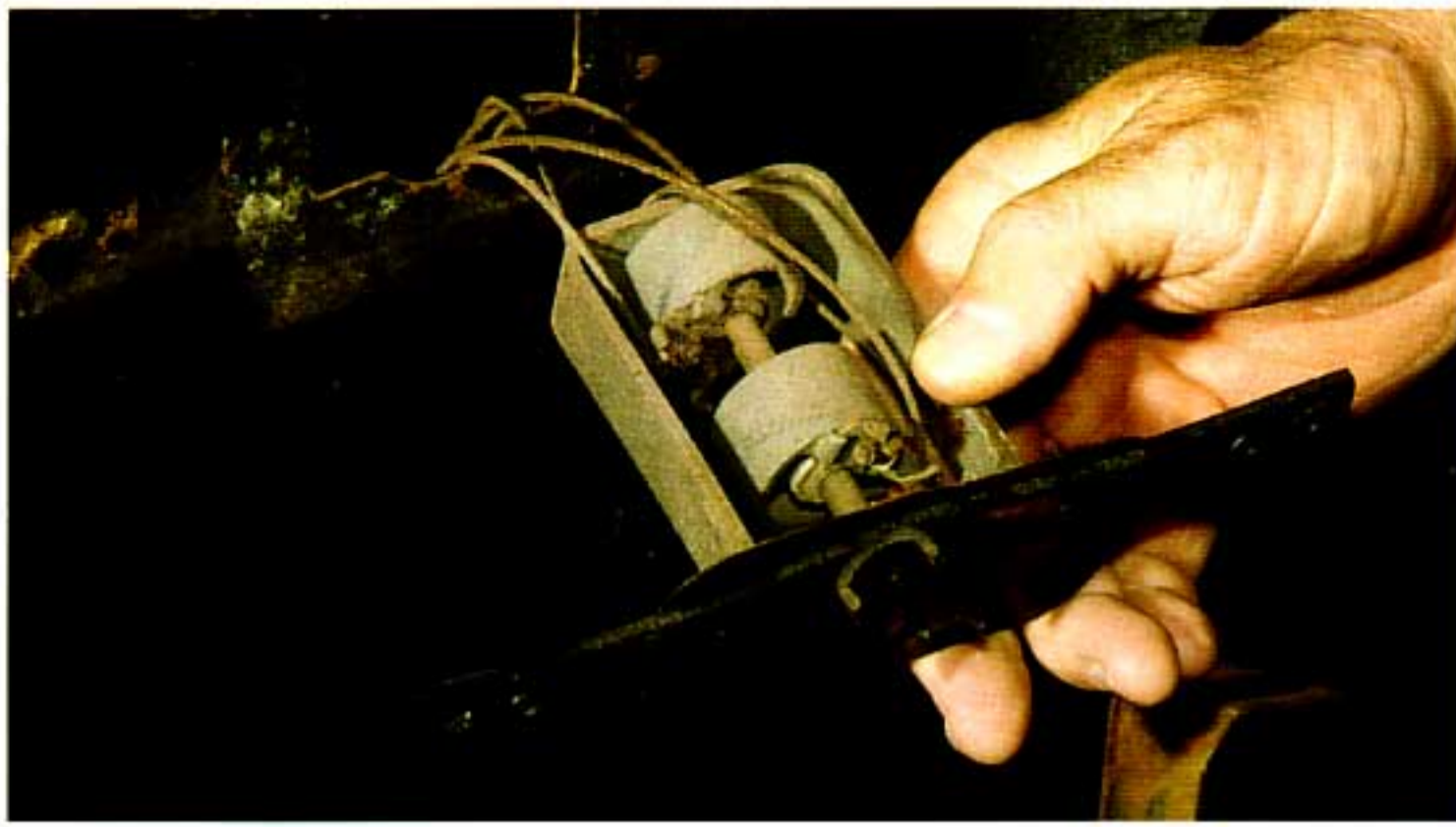
Photo #3: Each wiper transmission has two cables which attach to the center drum. The center drum is held to the fire wall with two #6 machine screws. Remove the two screws from the wiper drum and remove the wiper drum and wiper transmissions through the wiper drum hole.
