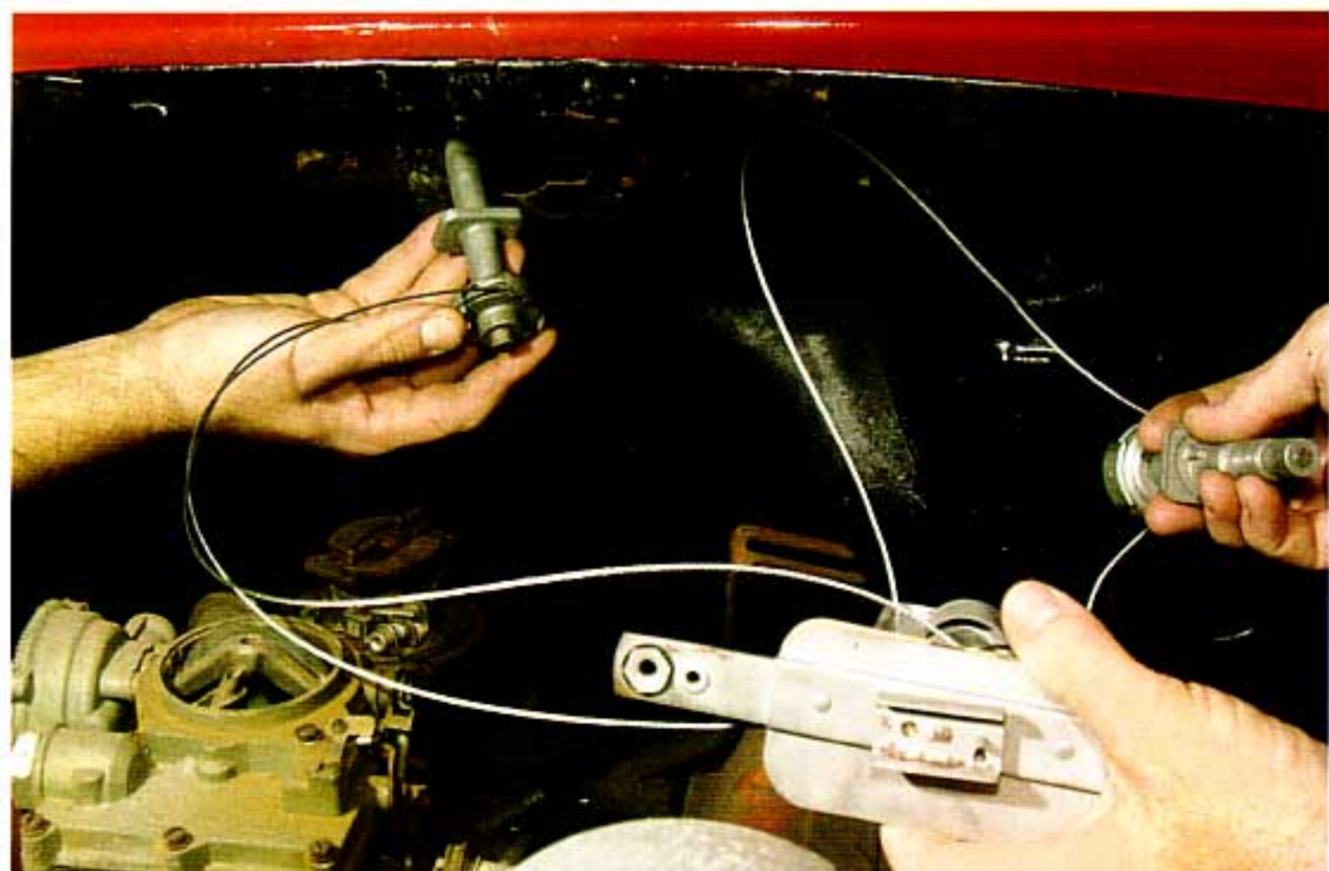
Photo #9: With the cables connected to the center drum, pass the wiper transmissions through the wiper drum hole from the engine side.
