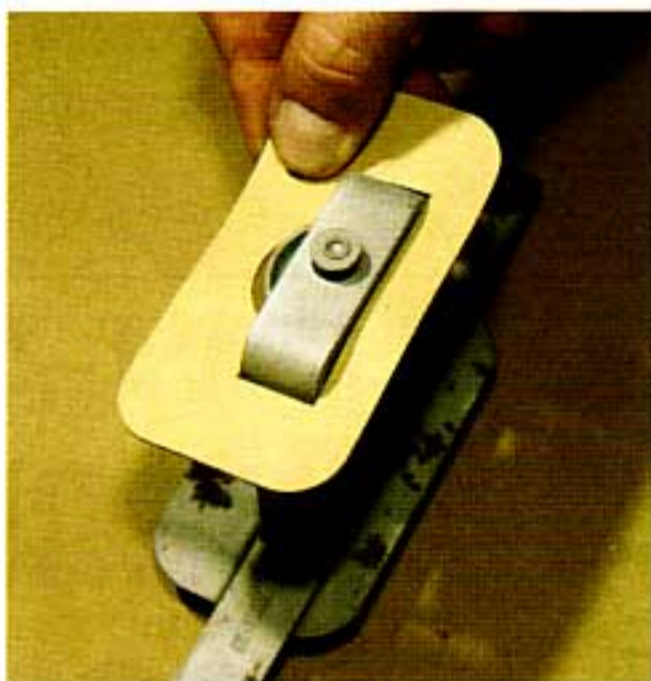
Photo #5: Before attaching the wiper transmission cables to the drum install a new seal part #05-20.
