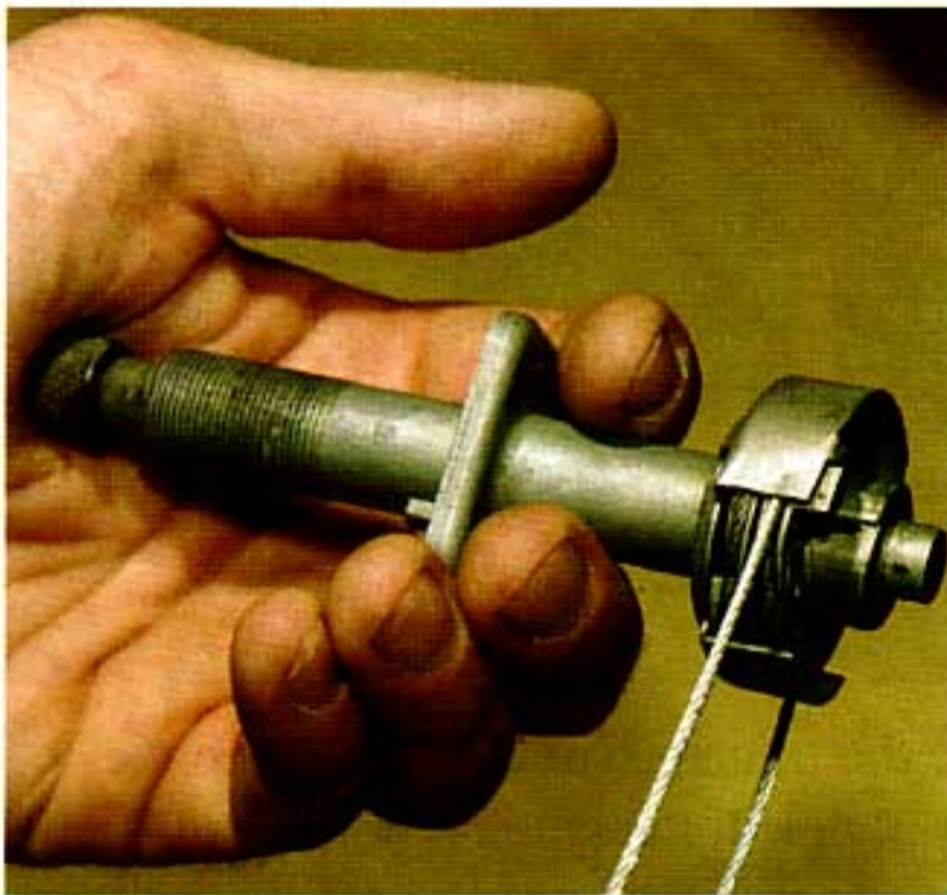
Photo #4: The length of the cables on wiper transmissions is fully adjustable. The cables on new transmissions must be adjusted all the way out before installing them in the car. To loosen the cables, depress the splined drum on the wiper transmission and pull both cables out evenly.
