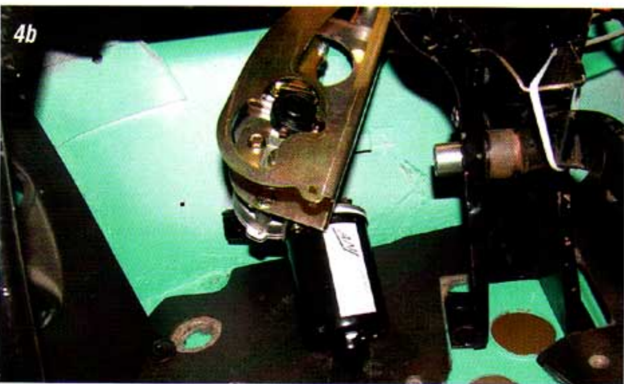
Photo #4a & 4b : The new wiper motor mounts to the left of the brake pedal assembly. The shaft on the wiper for the driver side wiper arm feeds through the cowl. The bent tab bolts to an existing hole in the firewall with a supplied 5/16" X 3/4" bolt and lock washer.
