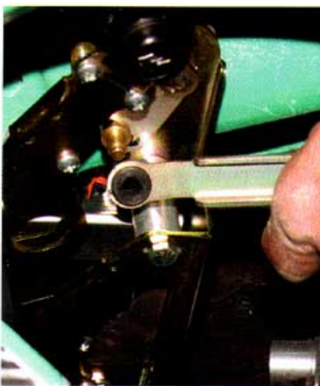
Photo #7: The linkage is held to the wiper motor with a flat washer and clip.
