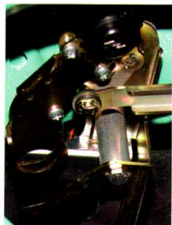
Photo #7: The linkage is held to the wiper motor with a flat washer and clip.
