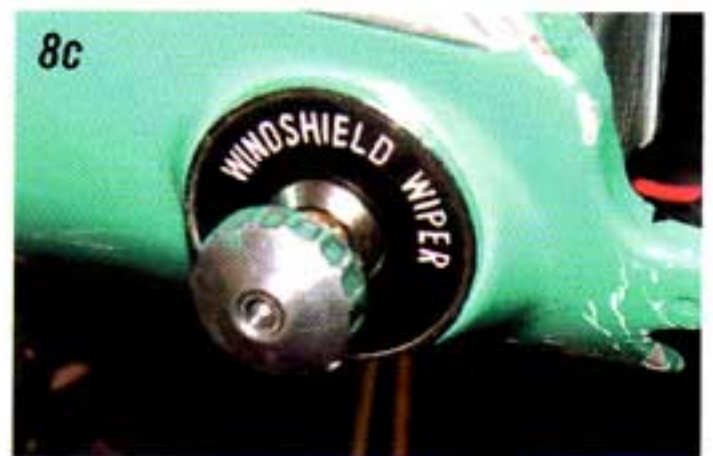
Photo #8a & 8b & 8c: The updated wiper system includes a new wiper switch. The switch will bolt in place of the original. The stock bezel and knob may be used.
