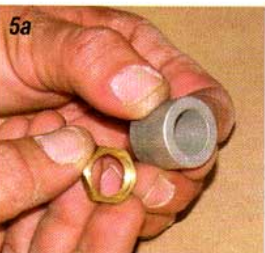
Photo #5a & 5b: There is a 1" long aluminum spacer and a brass nut that fits on the outside of the cowl. This holds the driver side transmission tight to the firewall. Make sure to use sealer under the aluminum spacers to seal the holes in the firewall.
