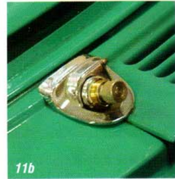
Photo #11a & 11b: The updated wiper kit still uses the stock wiper escutcheons. An escutcheon tool is included in the wiper kit.
