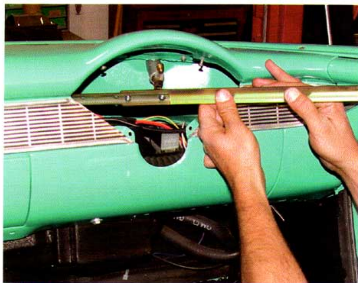
Photo #6: Feed the wiper transmission linkage through the speaker bezel opening on the passenger side.
