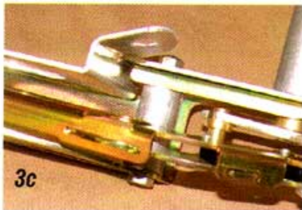
Photo #3a & 3b & 3c: There is a tab on the wiper motor that will need to be bent for the 1955 cars. Using two pair of vise grips or channel locks bend the tab up 30-degrees.
