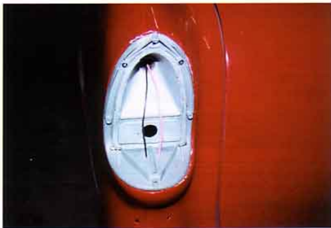
Photo #2a & 2b: Using your wire cutters, cut the two taillamp wires on each side of the car as close to the plastic connector as possible. Feed the wires back through the taillamp bulb hole in the housing. Using the scotch-lock type connectors provided with the kit, connect the black wire in the original harness to the black wire in the LED harness and connect the corresponding colored wires.
