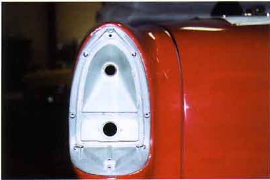
Photo #1a & 1b: Remove the original taillamp bezels and lenses. Remove the stock taillamp wiring from the housing by twisting the rubber boot and pigtail assembly turn counter-clockwise.
