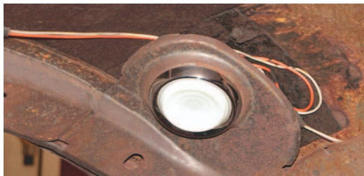
Photo #1: The 1955 Bel Air two-door hardtops and '55-'57 Nomads have two smaller dome lights located at the edges of the top. The other Tri-Five cars and '58-'60 non-Impalas have a larger dome light in the center of the top.
