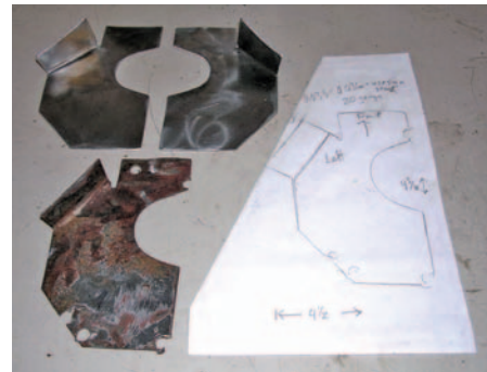
Photo #5: Plan to cut around the small braces that hold the bottoms of the kick panels. These will have to be removed from the old floor and welded to the new floor. The right side one was rusted to pieces, but the left one was in pretty good shape and served as a pattern to fabricate both sides in fresh 20 gauge metal.
