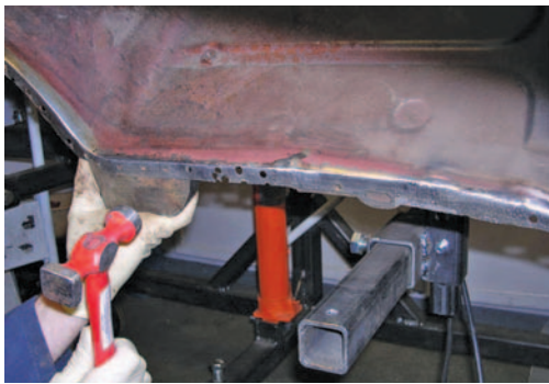
Photo #8: The flange was then cleaned of old seam sealer with lacquer thinner and straightened with a hammer and dolly.
