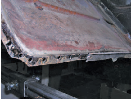
Photo #6: We used a reciprocating saw to cut out the old floor approximately one inch inboard of the original flanges. The old floor clearly had some issues!
