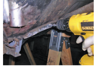
Photo #11: The new floor flanges were similarly prepped. They were sanded with 80 grit to remove the E-coating. Holes were punched along the top and bottom edges of the inner rocker that allow spot welding to the outer rockers later. All surfaces that were to be hidden inside welds were coated with weld-through primer. The body was then raised high on the rotisserie and the floor was placed on saw horses beneath it.
