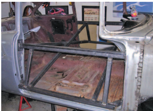
Photo #5: Plan to cut around the small braces that hold the bottoms of the kick panels. These will have to be removed from the old floor and welded to the new floor. The right side one was rusted to pieces, but the left one was in pretty good shape and served as a pattern to fabricate both sides in fresh 20 gauge metal.
