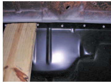
Photo #13: The rear flange was screwed to the trunk floor. This 2x6 plank provided a little extra persuasion to bring the floor flange up tight to the trunk flange.
