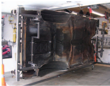
Photo #2: Once the body was on the rotisserie we could see all the body braces were rusty. In addition to several holes in the floor pans, the inner and outer rockers were full of holes as well. At this point we
