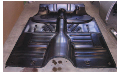
Photo #3: The new floor P/N 31-279 came with nearly everything we needed. Always have the new sheet metal on hand before cutting out the old!
