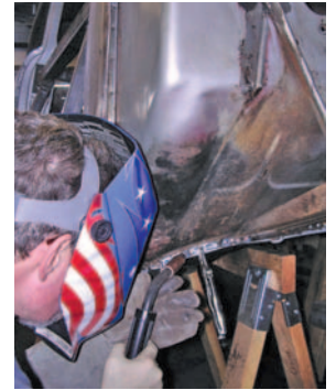
Photo #15: This is the almost finished project. Quite an improvement! The plug welds can be ground down until they look more like the factory spot welds if desired. Thanks to George Franklin #20000416 for the images and text. ✓
