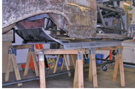
Photo #11: The new floor flanges were similarly prepped. They were sanded with 80 grit to remove the E-coating. Holes were punched along the top and bottom edges of the inner rocker that allow spot welding to the outer rockers later. All surfaces that were to be hidden inside welds were coated with weld-through primer. The body was then raised high on the rotisserie and the floor was placed on saw horses beneath it.
