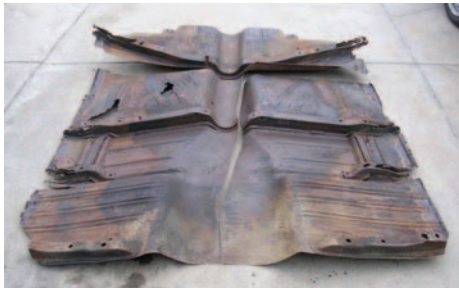
Photo #6: We used a reciprocating saw to cut out the old floor approximately one inch inboard of the original flanges. The old floor clearly had some issues!
