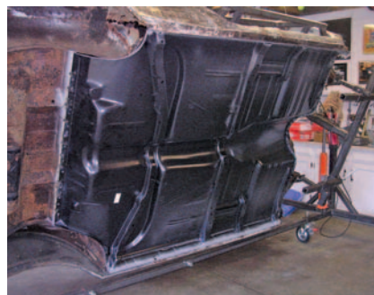
Photo #15: This is the almost finished project. Quite an improvement! The plug welds can be ground down until they look more like the factory spot welds if desired. Thanks to George Franklin #20000416 for the images and text. ✓
