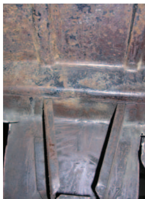
Photo #5: Plan to cut around the small braces that hold the bottoms of the kick panels. These will have to be removed from the old floor and welded to the new floor. The right side one was rusted to pieces, but the left one was in pretty good shape and served as a pattern to fabricate both sides in fresh 20 gauge metal.
