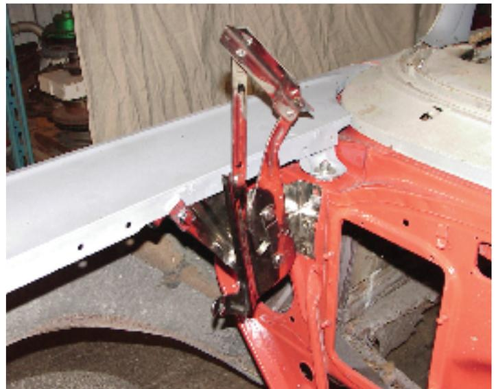
**Photo 3:** If you want to go that extra step, install the new polished stainless steel hood hinges P/N 54-31. With the new billet brackets and the stainless steel hinges, your '57 will look super custom under the hood! Good luck. ✓
