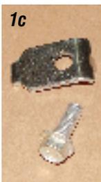
**Photos 1a, 1b & 1c:** The hood hinges on a 1957 Chevy have a pair of brackets that pinch the inner edge of the outer fender lip to stabilize side-to-side movement of the hinge. These brackets are bolted to the hood hinge with a 3/8" X 1" bolt on each side.
