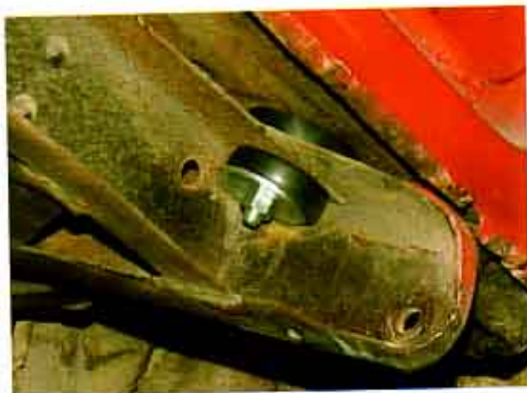
Photos #15a & #15b: The rear body mounts use 2 1/4" bolts with 1" washers under the head of the bolt and 1 7/8" washers. The bolts pass through from the trunk area.
