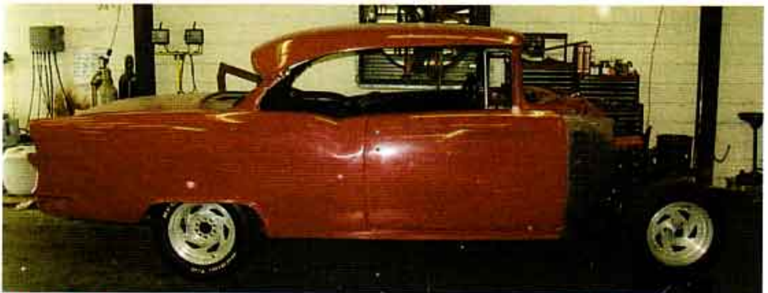
Photo #6: The car must be sitting on all four tires when replacing the body mounts to achieve proper door and fender alignment. The car can be on a drive-on lift or a set of jack stands under the rear end with a set of car ramps under the front tires.
