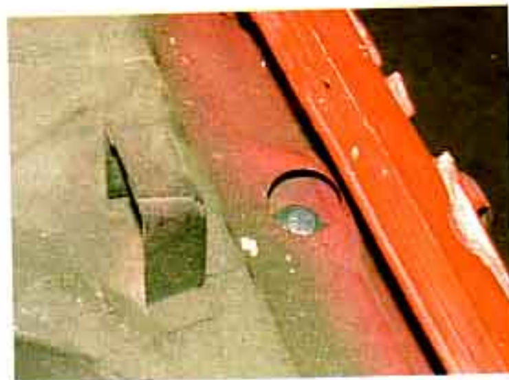
Photos #15a & #15b: The rear body mounts use 2 1/4" bolts with 1" washers under the head of the bolt and 1 7/8" washers. The bolts pass through from the trunk area.
