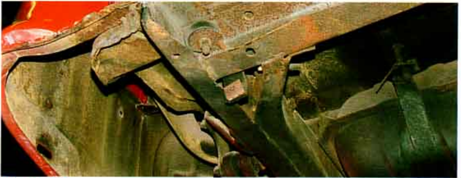
Photo #5: The eighth body mount is all the way to the rear of the frame. This mount bolts to the rear body support with a nut, bolt and washer.
