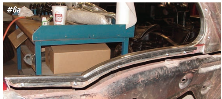
Photo #5a & 5b: The quarter window beltline moldings have a whisker strip stapled to the inner edge of the molding.
