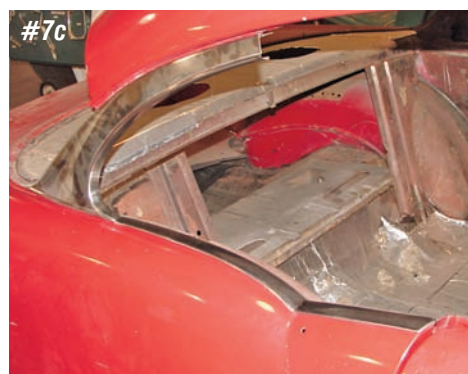
Photo #7a & 7b & 7c: The slots in the original beltline moldings are sometimes damaged. A new hole can be drilled in the molding and body to hold the moldings in place if needed.
