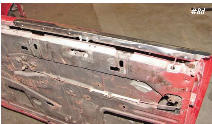
Photo #8a & 8b & 8c & 8d: The door window beltline moldings are held to the door with six #6 countersunk sheet metal screws included in kit P/N 34-38 . These outer door moldings do not receive whisker strips.
