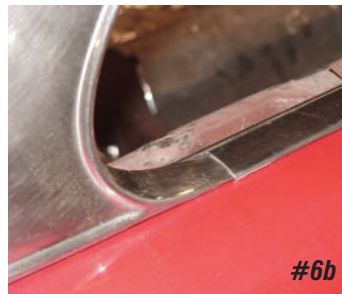
Photo #6a & 6b & 6c: The quarter window beltline moldings are held to the body with six #6 button head sheet metal screws kit P/N 34-113 . There are slots in the molding for front to rear adjustment.
