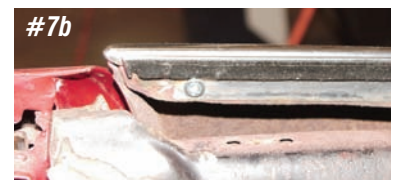
Photo #7a & 7b & 7c: The slots in the original beltline moldings are sometimes damaged. A new hole can be drilled in the molding and body to hold the moldings in place if needed.
