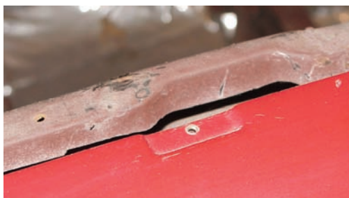
Photo #4a & 4b & 4c & 4d: At the front of the dogleg, there is a single hole. There is an impression in the top of the quarter panel that will match the hole in the dogleg. A #6 countersunk sheet metal screw, included in kit P/N 34-301 is used to hold the front of the molding in place. The rear tab on the dogleg is held to the body with a #6 counter sunk screw.
