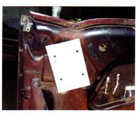
doors, install the new power regulators in through the access holes and guide the rollers into the glass and door tracks. Secure using the original holes and screws that attached the original regulators. Before installing the quarter regulators, drill two new holes using the template provided in the kit.
