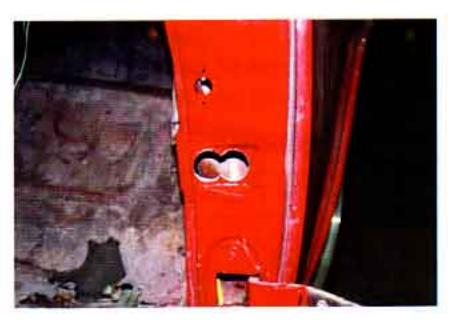
Photo #2a & 2b: The original cowl on 1955-58 cars has two small dimples that run horizontally just below the dome lamp switch area. If installing the original style conduits, pilot drill these holes with a 1/8" drill bit. Then drill the holes out to 1-1/2" using a hole saw. Using a flat file, connect the two holes so you have a nice oval opening in the cowl.
