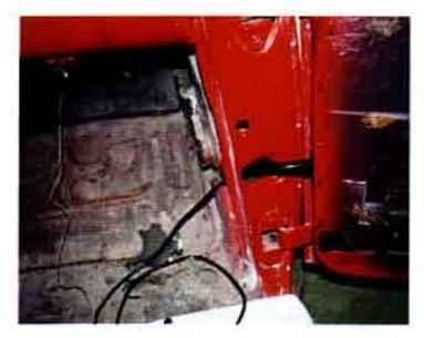
**Photo #6a & 6b:** Run the new wiring harness to all four window motors. Pass the front door wiring through the new conduits into the cowl area. Using the connectors provided, connect the corresponding color coded wires to each other to complete the wiring.
