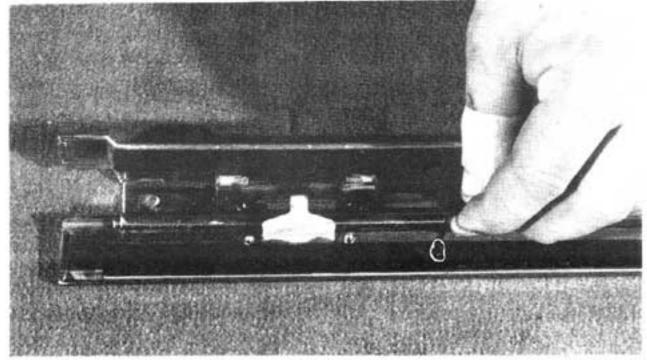
44. Slide the coiled end of the spring such that the two ends of the spring will go through their respective bracket retainers.
