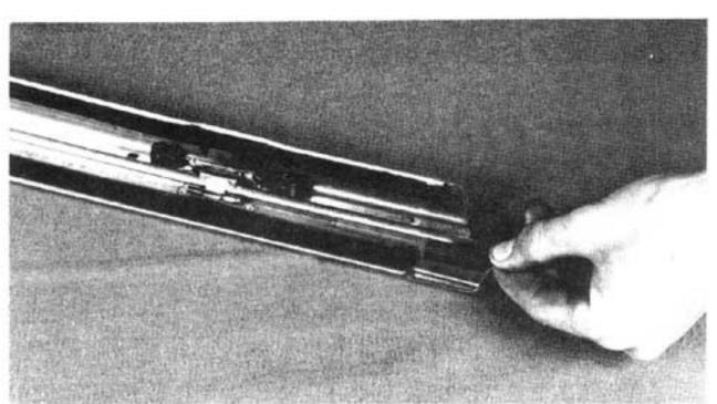
48. Using a small amount of 3M's Weatherstrip Adhesive, install the new forward flipper anti-chafe bumper. This rubber bumper helps protect the chrome of the vent window assembly. (If your kit does not contain a pair of these, they will be sent to you first-class mail as soon as we get them. These bumpers can be installed after the flippers have been reinstalled on the Coupe.) The restored flippers should not only look great, but should work great. 49. Reinstall the flipper onto the Hardtop.
