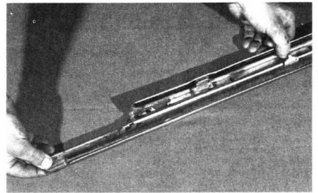
8. At this point, the two halves of the flipper assembly can be taken apart by sliding one end out of the other end. 9. You will notice that one part of the flipper is essentially flat and the second part of the flipper has a 90-degree bend. These will be referred to as the "flat part" and the "90-degree bend part." We suggest starting with the flat part of the flipper since it is the easier of the two. This will allow you to have some practice for the more difficult half of the flipper.
