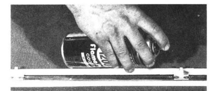
16. Using some masking tape, mask the stainless steel so that only the non-stainless steel metal strip and brackets will show. 17. The metal strip and brackets should be sprayed with a light, clear coat to protect the metal and to help prevent rust. VHT Clear, SP-115 (CCCI Part #30-62) is a good product for this purpose. 18. At this point, the stainless steel flat part of the assembly can be laid aside temporarily.
