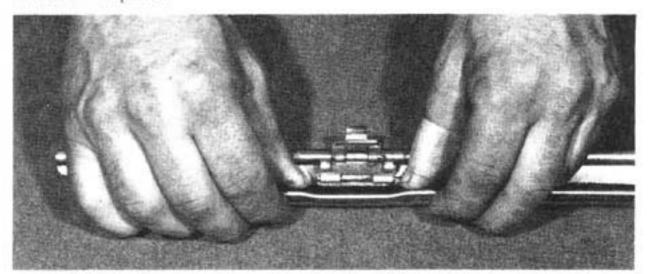
34. The very same procedure should be followed for the installation of the whisker strip on the 90-degree stainless steel flipper assembly. There is a 1¼-inch long dip in the whisker strip that needs to be formed as the installation with the adhesive is made.
