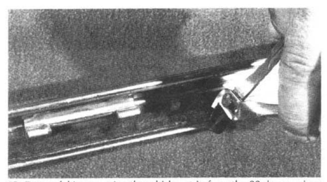
19. Be careful in removing the whisker strip from the 90-degree piece of the flipper. You will not use the flat-bladed screw driver in the same manner as you did for the flat piece. A pair of diagonal cutters can be used to "roll" the old whisker strip out from under the stainless steel lip which retains the whisker strip. If by some chance the old whisker strip bead tears off and remains under the lip, you will need to remove
