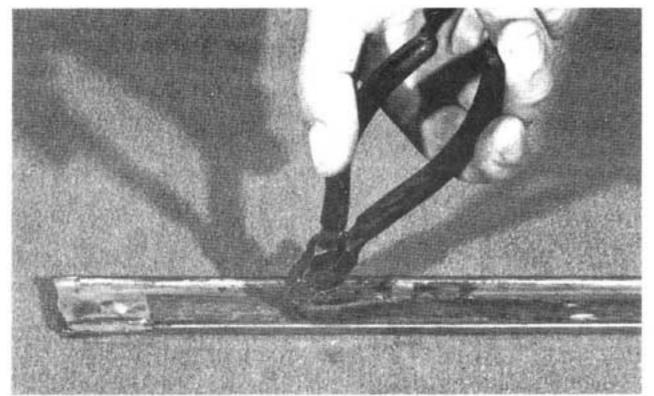
11. Using a pair of diagonal cutters, grab the end of the whisker strip and gently pull the whisker strip out from under the pinched lip of the stainless edge of the flipper. 12. Once the end of the whisker strip is started, grab the bead that was under the lip and begin to "roll" it out from under the lip. The rustier the whisker strip, the harder it is to remove.
