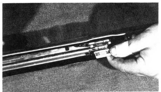
47. Install the brand new nylon bumper over the metal tab that acts as the closer for the flipper.
