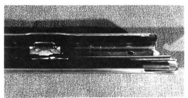
38. Reinstall the retaining pin for the flipper "closer." The head of the pin is towards the closest end of the flipper. 39. Rebend the end of the pin slightly, such that the pin will not slide out of the bracket.
