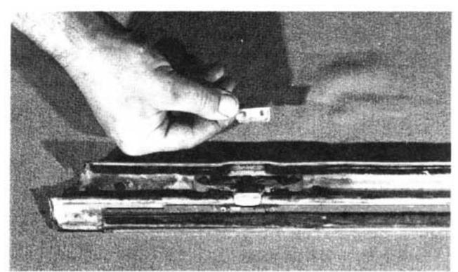
Remove the flipper. (For specific information on the removal and reinstallation of the Hardtop flipper, see the Tech Article in the the Restoration section pg 17.)
