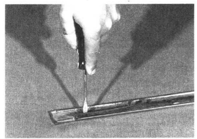
10. Using a flat-bladed screw driver, start bending the whisker strip up away from the stainless steel. Don't use too much pressure. We cannot emphasize enough that taking time and using a lot of patience in this step of the restoration is very important. A set of nice flippers are not easily replaced.
