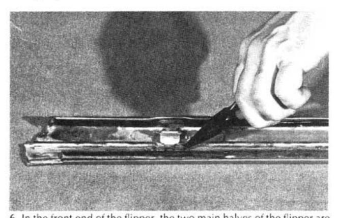
6. In the front end of the flipper, the two main halves of the flipper are secured together with a pin in the closing assembly. The end of this pin is usually bent slightly so that it will not work itself out of the assembly. Straighten this pin with a pair of pliers. 7. Slide the retaining pin out of the closing assembly.
