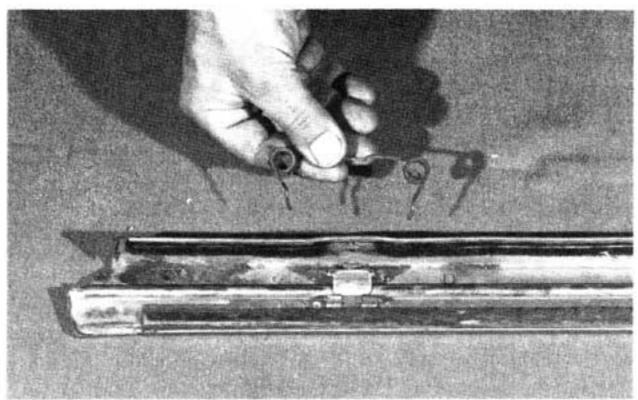
Using a pair of needle-nosed pliers, slip the two ends of the doublecoil spring out from under the retaining tabs on the closer hinge. Remove the spring from the assembly.
