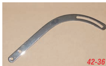
Photo 1: The original generator bracket was bolted to the side of the exhaust manifold forward of the #1 exhaust port with two 3/8" bolts and lock washers.
