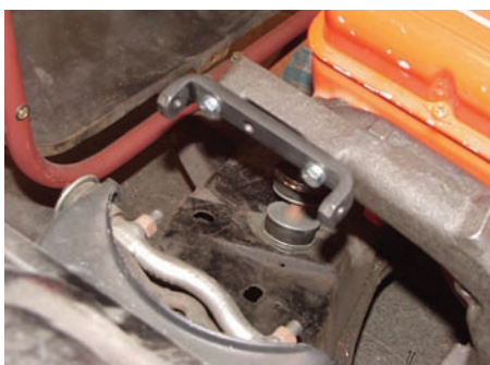
Photo 1: The original generator bracket was bolted to the side of the exhaust manifold forward of the #1 exhaust port with two 3/8" bolts and lock washers.
