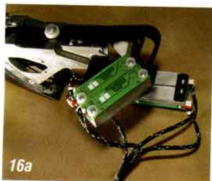
Photo #16a, 16b & 16c: Plug the wiring harness into the control panel and pass the unit through the glove box opening and back through the dash heater control opening. Install the face plate and knobs, secure the control panel to the dash. Attach the other end of the control panel wiring harness to the plug on the ECU module on the passenger side top of the evaporator. Also plug in the lead from the blower motor to the ECU.
