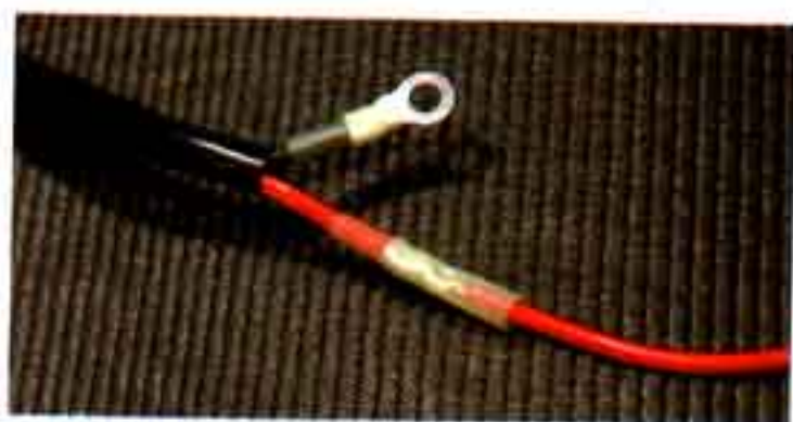
Photo #34: The red wires in the harness connect to the red lead wires on the fans. The black wires from the fans should be connected to a good ground.
