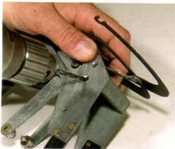
Photo #3a & 3b: Using a 1/8" drill bit, remove the original rivets that secure the upper rear cable bracket to the panel cage and discard the bracket. Install the new slider switch bracket using the two #6-32 machine screws and nuts provided.
