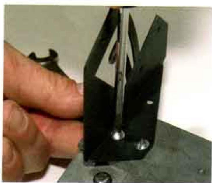
Photo #3a & 3b: Using a 1/8" drill bit, remove the original rivets that secure the upper rear cable bracket to the panel cage and discard the bracket. Install the new slider switch bracket using the two #6-32 machine screws and nuts provided.
