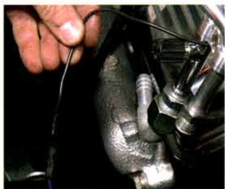
Photo #38a & 38b: The blue wire from the evaporator under the dash needs to be connected to one of the terminals on the binary switch on the liquid line. The other terminal on the binary switch connects to the compressor with the supplied wire.
