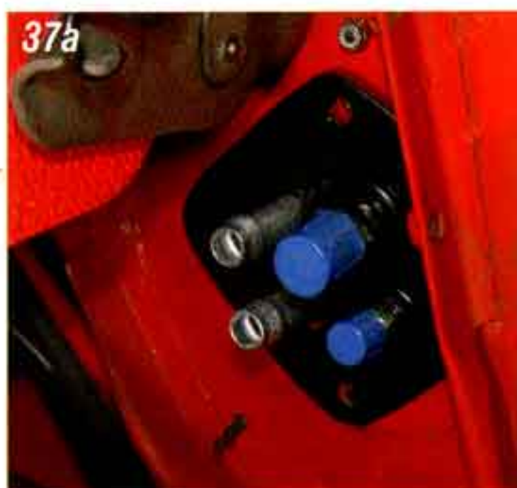
Photo #37a & 37b: The small fitting on the underdash evaporator unit is the liquid line
