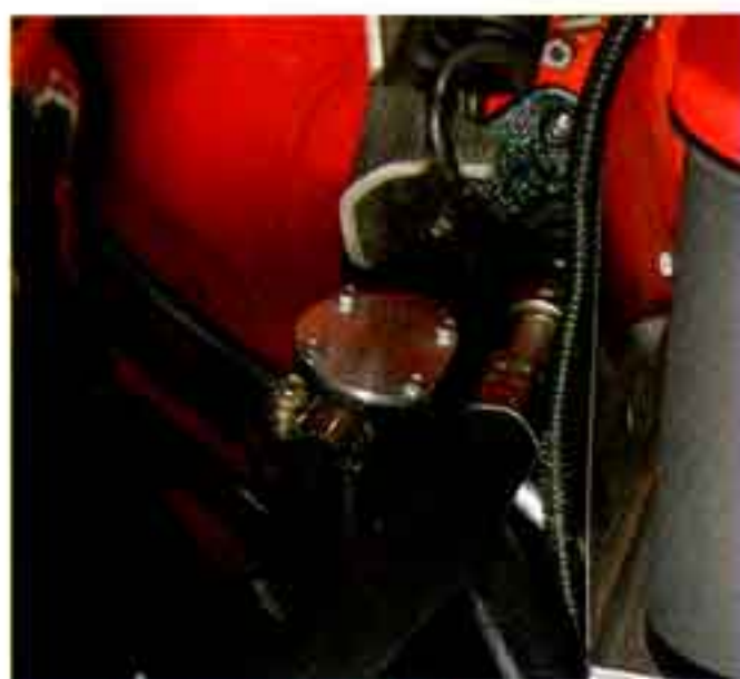
Photo #39a & 39b: The larger fitting from the evaporator attaches to the larger fitting on the compressor using the #10 hose with the straight fitting on one end and the 90-degree fitting on the other. The small fitting on the compressor connects to the large fitting on the condenser using the #8 hose with the 45 degree fitting on each end.
