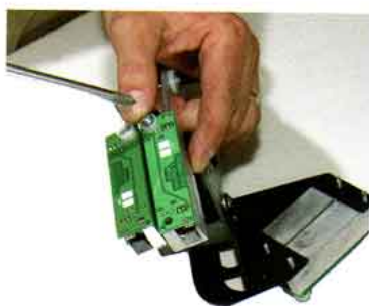
Photo #4a & 4b: There are four identical slider switch PC boards and cast metal holders. These assemblies attach to the control panel and will control the computer ECU on the air unit. Attach two of the assemblies to the new slider switch bracket. Make certain the loop ends of the new control levers engage the levers on the slider switches. If the levers drag on the sides of the metal holders, slightly bend the levers in or out until proper clearance is achieved. Secure the assemblies with the #8 x 1-1/4" self-tapping screws and nylon cupped washers. Tighten the screws until they are just barely snug. Do not over tighten or the PC boards may be damaged.
