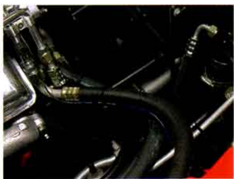
Photo #39a & 39b: The larger fitting from the evaporator attaches to the larger fitting on the compressor using the #10 hose with the straight fitting on one end and the 90-degree fitting on the other. The small fitting on the compressor connects to the large fitting on the condenser using the #8 hose with the 45 degree fitting on each end.
