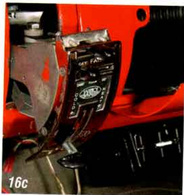
Photo #16a, 16b & 16c: Plug the wiring harness into the control panel and pass the unit through the glove box opening and back through the dash heater control opening. Install the face plate and knobs, secure the control panel to the dash. Attach the other end of the control panel wiring harness to the plug on the ECU module on the passenger side top of the evaporator. Also plug in the lead from the blower motor to the ECU.
