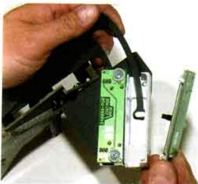
Photo #4a & 4b: There are four identical slider switch PC boards and cast metal holders. These assemblies attach to the control panel and will control the computer ECU on the air unit. Attach two of the assemblies to the new slider switch bracket. Make certain the loop ends of the new control levers engage the levers on the slider switches. If the levers drag on the sides of the metal holders, slightly bend the levers in or out until proper clearance is achieved. Secure the assemblies with the #8 x 1-1/4" self-tapping screws and nylon cupped washers. Tighten the screws until they are just barely snug. Do not over tighten or the PC boards may be damaged.
