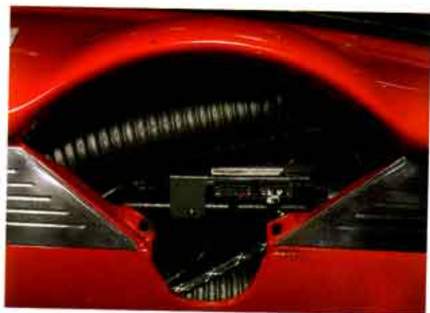
Photo #15: Using the same procedure for the routing large diameter duct hose, run the smaller duct hose from the top of the evaporator to each of the dash defroster outlets.
