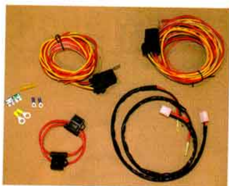
Photo #32a & 32b: The fan wiring harness kit includes two short leads with a red and black wire that plug into the electric fans. This will allow you to unplug the fans and remove them if you ever need to.
