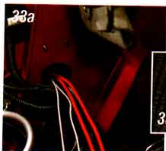
Photo #33a, 33b & 33c: The relays for the electric fans can be mounted anywhere on the car. We mounted ours up under the dash to keep the engine compartment nice and clean. The two red wires and two gray wires from the relays need to be routed out to the electric fans. The yellow wire on the relay needs to be connected to full-time 12-volts. The orange wire should be connected to ignition on 12-volts. The two gray wires should be butt connected together and connected to the temperature sender on the radiator.
