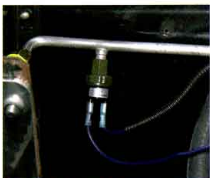
Photo #38a & 38b: The blue wire from the evaporator under the dash needs to be connected to one of the terminals on the binary switch on the liquid line. The other terminal on the binary switch connects to the compressor with the supplied wire.
