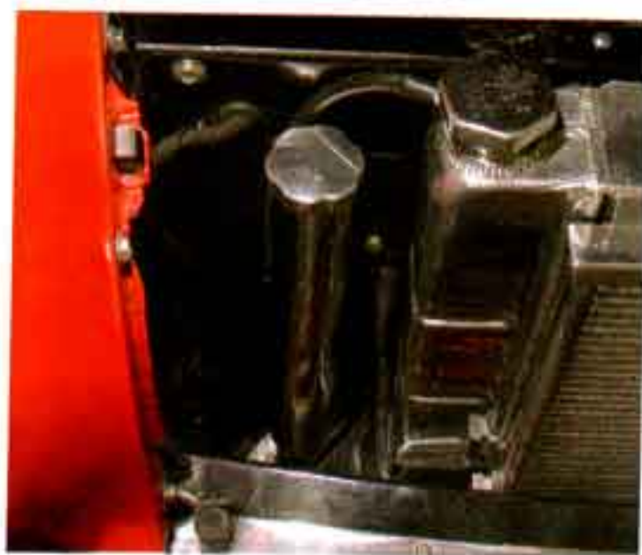
Photo #36: Once the radiator and condenser are in place, the grille can be reinstalled. This is where it gets tight on 1955-56 cars. The hood latch striker plate and support need to be trimmed to give enough clearance with the condenser.
