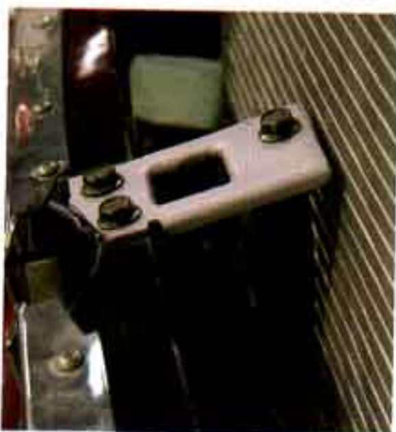
Photo #36: Once the radiator and condenser are in place, the grille can be reinstalled. This is where it gets tight on 1955-56 cars. The hood latch striker plate and support need to be trimmed to give enough clearance with the condenser.
