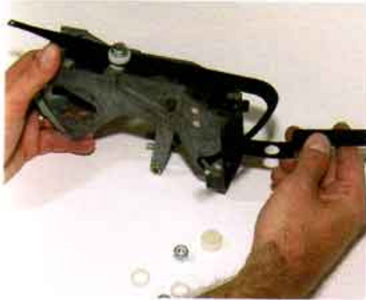
Photo #2: Install the two new horizontal blower and mode levers from the kit using the 5/16" bolt, washers, nylon spacers and nut provided.
