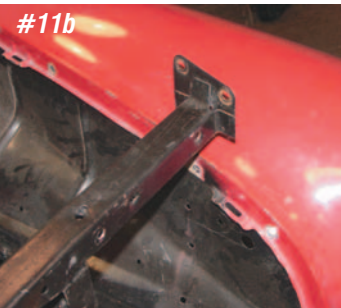
Photo #11a & 11b & 11c & 11d: Remove the two bolts on each side of the core support where it is bolted to the front fenders. There are often shims between the core support and inner flanges of the fenders.
