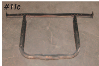
Photo #11a & 11b & 11c & 11d: Remove the two bolts on each side of the core support where it is bolted to the front fenders. There are often shims between the core support and inner flanges of the fenders.
