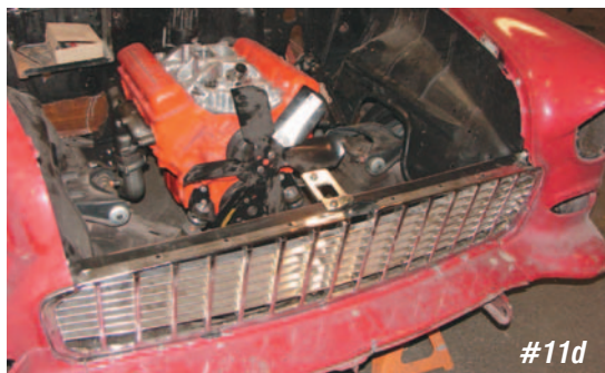
Photo #11a & 11b & 11c & 11d: Remove the two bolts on each side of the core support where it is bolted to the front fenders. There are often shims between the core support and inner flanges of the fenders.
