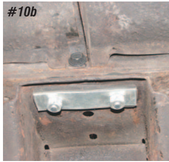
Photo #10a & 10b: The radiator core support is bolted to the frame in the center with two 3/8" carriage bolts and nuts. There are cushions and shims located here between the core support and frame.
