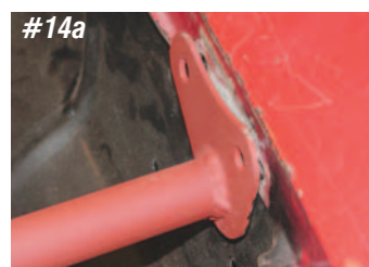
Photo #14a & 14b & 14c: The tubular core support bolts to the fenders using the same holes the stock core support uses. Shim as required using the supplied new shims.
