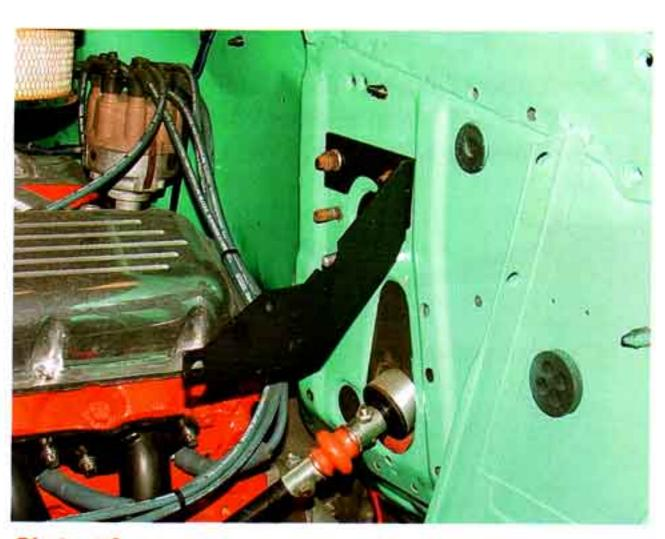
**Photo #2:** If you are installing the non-power system, you can leave the original pedal clevis and pushrod in place. Install the proportioning valve bracket using the upper two master cylinder studs on the firewall.
