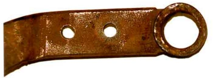
Photo #7: If you are installing a power dual master cylinder system, the original brake pedal clevis and rod will need to be removed from the swing pedal under the dash. For proper pedal travel with a power system, a new 3/8" hole should be drilled in the brake pedal swing arm 1" below the original hole. This is easier to do if the pedal is removed from the car.
