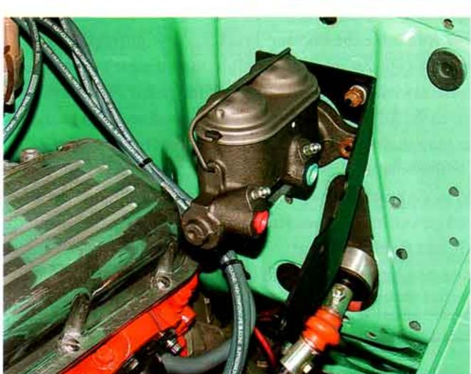
Photo #3a & 3b: It is helpful to bench bleed the master cylinder by adding fluid and pumping while it is chucked in a vise. Pump the cylinder until it is free of air and fluid is running out both lower ports. Install the dual master cylinder using the two lower studs on the firewall. Be sure the pushrod engages the hole in the piston at the rear of the master cylinder.
