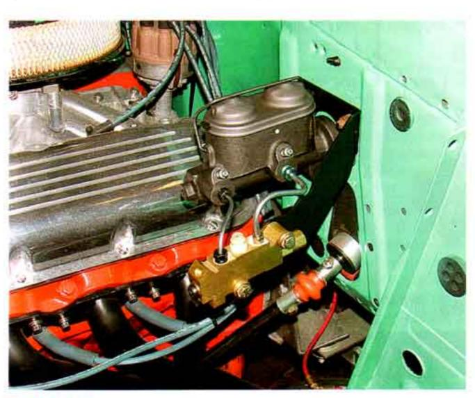
**Photo #4:** Install the proportioning valve on the bracket with the large port fitting facing the rear. Install the two lines between the master cylinder and the proportioning valve.
