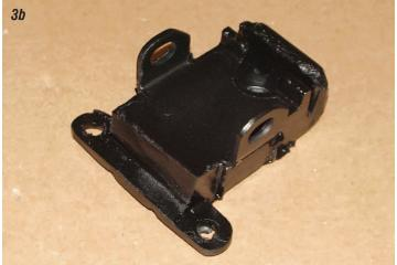
**Photos 3a, 3b & 3c:** If the side engine mount kit on your car uses the heavy duty style GM mount, the driver's side mount will need to be trimmed to clear the header. Using a hack saw, band saw or cut-off wheel, simply trim the upper support plate and excess rubber from the side engine mount on the driver's side. A little black paint and the heavy duty motor mount will look like a stock non-heavy duty mount and will now clear the header tube just fine.
