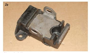
**Photos 2a & 2b:** Other brand side engine mount conversion kits use the early model Chevy Nova, Chevelle or Camaro GM-style engine mounts. These mounts work fine except the driver's side header tubes on the **P/N 24-53** and **24-53C** headers are tucked in
