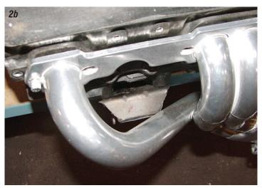
so tight to the engine block to clear the various steering applications that it will interfere with the upper support plate on a heavy duty style GM motor mount.
