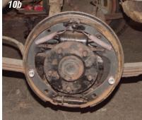
**Photos 10a & 10b:** Before installing the axle into the rear end, lubricate the O-
