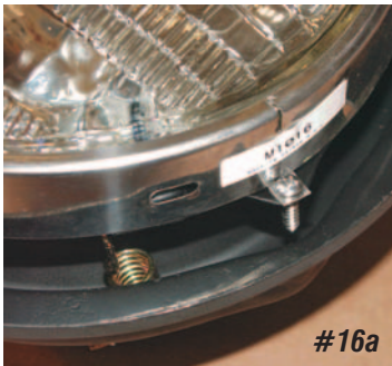
Photo #16a & 16b: The trim ring for the headlight is held to the sub bucket with three small sheet metal screws. Key the headlight and sub bucket assembly into the new adjuster screws and snap the spring into the hole in the ring using needle nose pliers.
