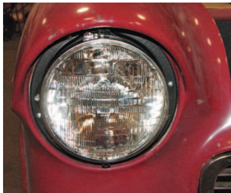
Photo #16a & 16b: The trim ring for the headlight is held to the sub bucket with three small sheet metal screws. Key the headlight and sub bucket assembly into the new adjuster screws and snap the spring into the hole in the ring using needle nose pliers.
