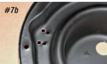
Photo #7a & 7b: New holes must be drilled for the new adjuster brackets. Using the original holes as a guide, line up the new bracket to the outside of the original holes and mark the bucket where the new holes need to be drilled. Drill two 3/16" holes for the new mounting hardware.
