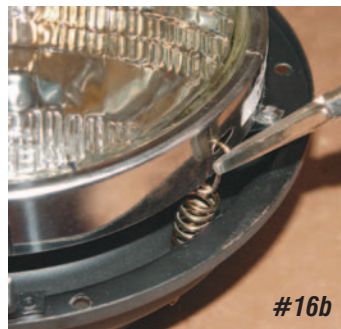
Photo #16a & 16b: The trim ring for the headlight is held to the sub bucket with three small sheet metal screws. Key the headlight and sub bucket assembly into the new adjuster screws and snap the spring into the hole in the ring using needle nose pliers.
