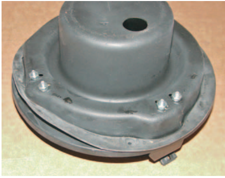
Photo #14: The headlight bucket seals P/N 05-15 for 1955-56 and P/N 05-53 for 1957 will match the contour of the bucket and fit between the bucket and fender.
