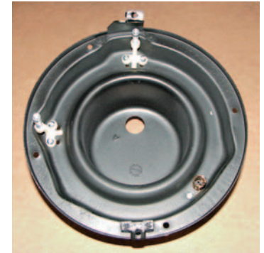
Photo #10: The refurbished bucket is now ready to go back in the car. It's always fun to take a damaged original part and with a little time and money bring it back to something that will last another 50 years!
