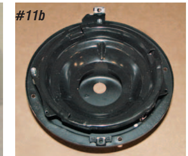
Photo #11a & 11b: The original sub bucket has two ears that will key into the grooves on the adjuster screws. If your sub buckets and rings need to be replaced, order P/N 28-09.
