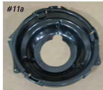
Photo #11a & 11b: The original sub bucket has two ears that will key into the grooves on the adjuster screws. If your sub buckets and rings need to be replaced, order P/N 28-09.
