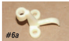
Photo #6a & 6b: The replacement adjuster brackets included in kit P/N 34-100 are made of nylon and attach to the headlight bucket using the supplied hardware. There is a tail on the replacement bracket that must be removed for this application. Using a pair of side cutters, remove half of the tail.
