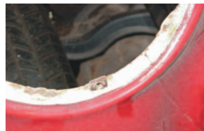
Photo #13: There are four J-nuts at the front opening of the fender for the headlight bucket retaining screws. These new nuts are supplied with the hardware kit.
