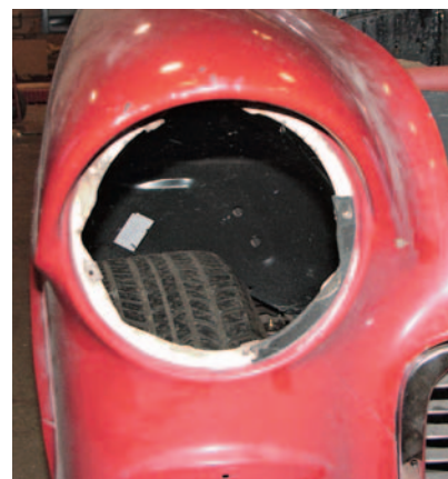
Photo #12: A flat rubber seal fits between the headlight bucket and the front fender. When you removed the bucket from the fender, the seal was probably not there or was dried up and broken. We will replace these seals.
