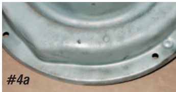
Photo #4a & 4b: Using the grinder, grind off the head of the rivet for the sub bucket spring and drive the rivet out.
