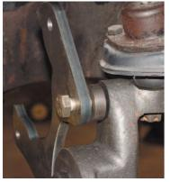
*Photo #7:* Install the new dropped spindles on the ball joint studs and secure with the ball joint nuts and new cotter pins. Install the coil springs and shocks. If you desire a 4" drop, this is the time to install 2" lowering coils **P/N 21-133**.
