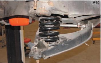
*Photos #4a, #4b & #4c:* Remove the upper and lower ball joint cotter pins and nuts and using a ball joint splitter, remove the spindle from the ball joints.
