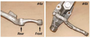
*Photos #6a & #6b:* The boss on the steering arm is thicker at the rear thus the need for the longer stud. The arm will be held to the spindle with 7/16" lock nuts supplied with the dropped spindles.
