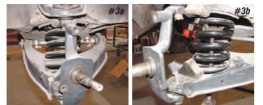
*Photos #3a & #3b:* Once the spindle is stripped of all parts it can be removed. Before removing the spindle, a coil spring compressor must be used to take the load off of the control arms. First remove the shock absorber and feed the coil spring compressor up through the hole in the lower control arm and compress the spring so that there is no load on the control arms.
