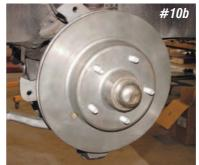
(also included in the brake kit) from an early GM "A" Body. Pack the wheel bearings with good quality grease. Install the bearings, inner seal, spindle nut and washer, cotter pin and dust cap.
