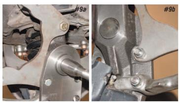
**Photos #9a & #9b:** The lower ear on the caliper bracket attaches to the spindle using the 7/16" hole above the rear steering arm stud. A 7/16" x 1-1/2" bolt and lock nut secures the bracket to the inside face of the spindle.
